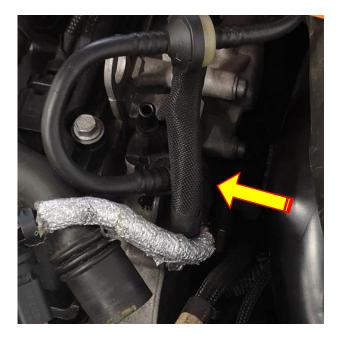
14. Pull the vac line off the vac pipe, you can see the black vac pipe arrowed below. Take the supplied brass T piece and push it into the OEM vac tube as shown in the image below.
