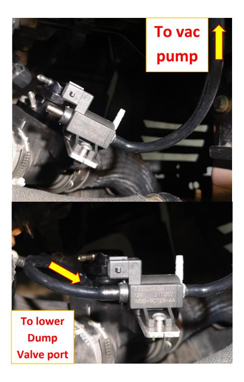
27. Connect the end shown on the supplied wiring loom to the solenoid as shown in the image below.
