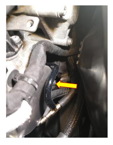
16. Cut a long section of supplied vac line and connect one side to the T piece to seal it off. This vac line will be running to the valve so leave this long for now as you can cut it back in a later step. Use the supplied cable ties to secure all 4 vac line points (one to OEM vac pipe at vac pump, and one for each vac line on the T piece)
