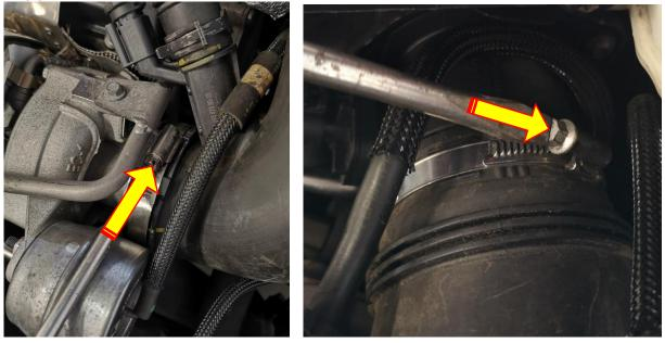
7. Pinching your fingers on the flat areas of the clips will remove the two breathers from the right-hand side of the inlet pipe
