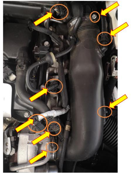
6. Using a flathead screwdriver or a 7mm socket and suitable drive undo the two hose clamps attaching the inlet pipe to the turbo and airbox
