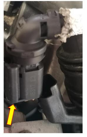
**11**. Using a hose clamp removal tool or long nose pliers loosen the hose clamp from the base of the plastic, over the ribbed section and place it on the tube as shown in the image below
