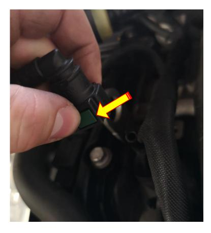
9. Push the lock to the clip and pull from the plastic **NEVER THE WIRES** to disconnect the sensor below from where the inlet pipe meets the airbox
