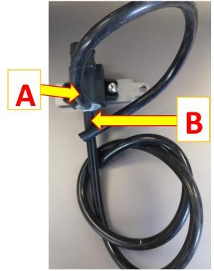
25. With a 5mm allen key undo the OEM bolt shown place the solenoid and bracket into position and tighten the bolt back up allowing it to still move with relative freedom. This is so that you can shift the solenoid around when fitting the vac lines
