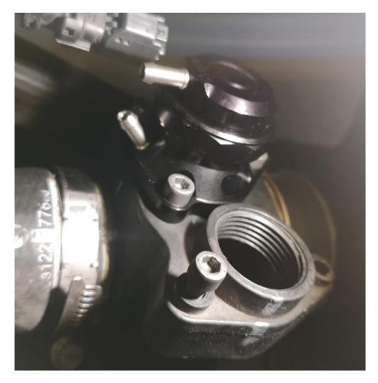
23. Using a 3mm allen key tighten the two bolts to secure the solenoid to the plate in this orientation.
