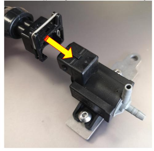
28. Connect the other end. Look for the hole on the OEM loom as this is where the small pin on the supplied loom will engage into.
