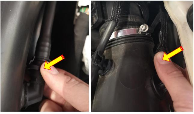
8. Push the green clips into the vac pipe that is situated on top of the vac pump to disconnect it
