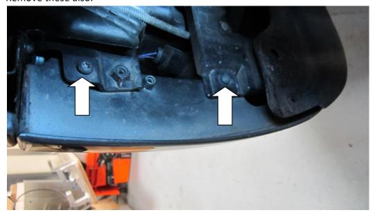
6. Located behind this panel where the bumper meets the arch are two 10mm fasteners, remove the 10mm nuts that hold the sides in place.
