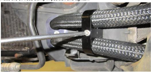
35. Using the P clips provided place them into position on the longer of the two oil lines, use the two M6 x 16 cap screws with M6 nuts and washers.
