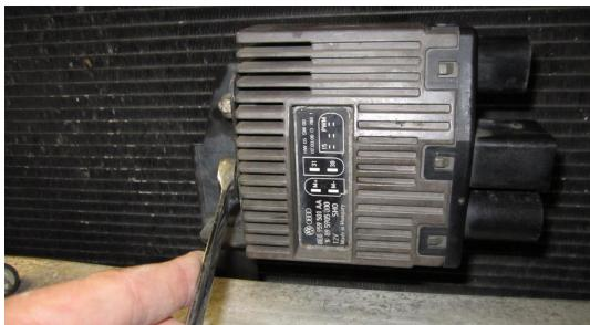
18. Remove the bracket that held the control unit in place, use a 10mm spanner on the hex heads located on the rear of the crash bar.
