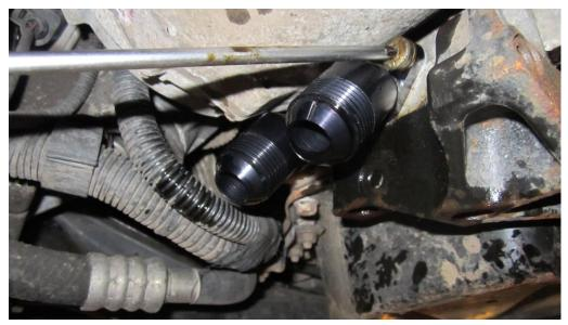
28. Slide the oil cooler assembly under and behind the crash bar into position.
