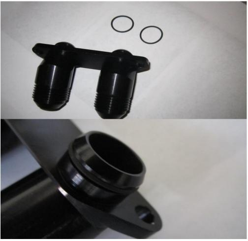
27. You can now install the sandwich plate to the engine. Put into position and use the two bolts you removed in section 12 to fix in place.
