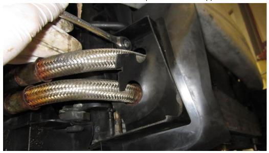
15. Now you will be able to slide out the cooler from between the radiator and the power steering cooler.
