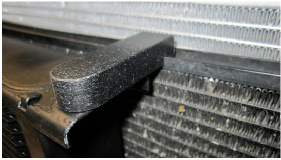
41. Using the four M6 x 10mm button heads and washers mount and tighten the blocks using a 5 mm Allen key.
