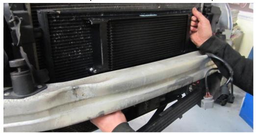
29. Using the two M6 hex heads removed in section 18 that held the fan controller bracket in position, attach the new assembly and tighten using a 10mm spanner.
