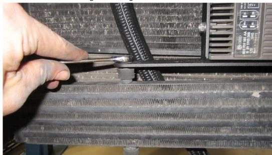
31. Feed the oil lines towards the left hand side of the vehicle when viewed from the front and through the slam panel towards the sandwich plate. Push the oil lines through where arrowed.
