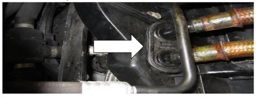
17. The fan controller can also be removed now. Undo the three wiring harnesses then remove the 10mm nuts holding on the control unit.
