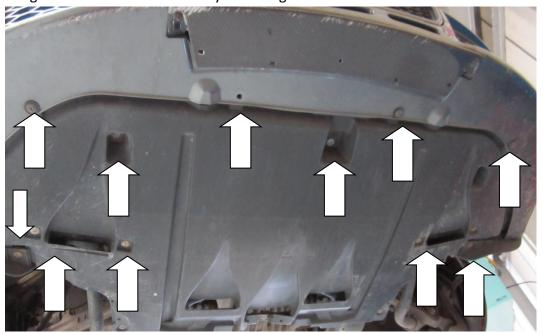
3. Using a T30 torx driver, undo the fasteners pictured. They are towards the rear of the under tray in the corners.
