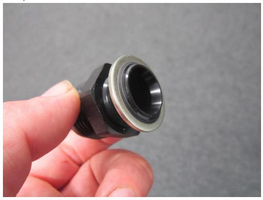
21. Now attach the M22 to dash 12 adaptor to the oil cooler, and using an adjustable spanner (or -12 spanner) tighten them down.
