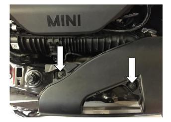
Undo the 1x screw using a T25 Torx driver. Push the wiring clip downwards using a flatblade screwdriver or similar tool to remove it. The next part may require two people to hold the plastic catches apart while the other removes the MAP sensor. Lift the bonnet and begin by removing the intake scoop, this will give better access while carrying out the installation. Undo 2x 10mm nuts and unclip at the airbox.
