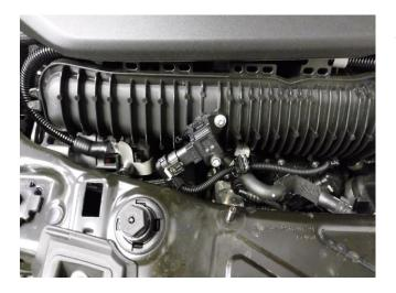
The boost tap will be fitted on an angle if you have the later inlet manifold, as shown in the picture.
