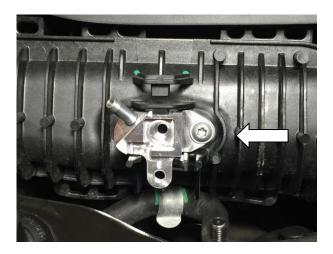
Refit the MAP Sensor to the boost tap, lubricate the O-ring with silicone spray and secure with the M6x16mm Allen cap bolt supplied. You can then attach the hose from your boost gauge to the takeoff nipple on the block. Refit the intake scoop. Ensure the O-ring supplied is fitted to your boost tap. Lubricate with a silicone spray before fitting to the manifold. Push the boost tap firmly into position and secure with the OEM screw.
