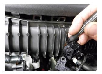
If you have a later vehicle fitted with this inlet manifold, you will have to file one of the plastic fins to allow the boost take off to fit. Just offer up the boost tap and mark the area on the fin that needs filing down, then use a file or blade to remove the excess material.
