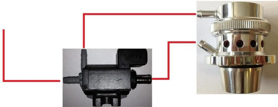
7. Take the solenoid and large cable tie provided and secure it to the large wiring loom next to the airbox vacuum pipe. Take the wiring loom supplied in the kit and connect it to the solenoid and the other end to the loom which was attached to the OE valve.
