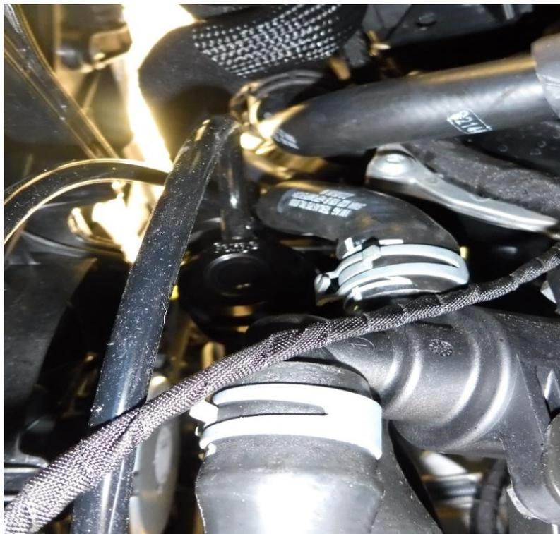
6. The next set of pictures are for illustration purposes - they may not be representative of your engine, but they are the clearest way to show you how to connect your solenoid to the atmospheric or recirculating valve you have fitted. Use the supplied silicone hose to do this, use a sharp knife or side cutters to cut the hose to length.
