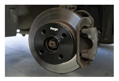
Fit the wheel and torque the wheel bolts to the required setting and follow these steps for the remaining spacers.
