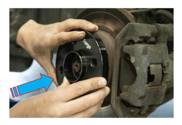
Place the new spacer onto the disk, line up the holes for the wheel bolts.
