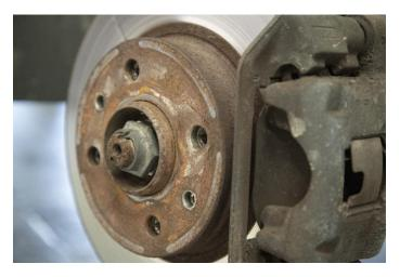
Give the mounting surface and centre bore of the disk a clean with a wire brush before fitting the Forge Motorsport spacers.
