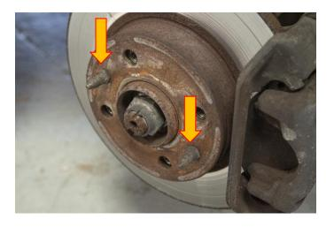
Jack the vehicle up and remove the wheel and locate the two bolts attaching the disk to the hub.
