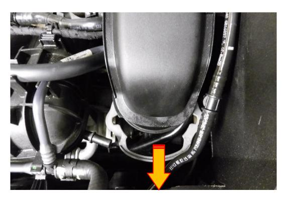
5. Remove the factory O-ring seal from the coupler on the OE boost inlet pipe and place it on the charge cooler inlet pipe.
