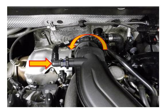
4. With the use of a flat blade screwdriver or trim tool, release the plastic retaining clip which holds the other end of the boost inlet pipe. The boost pipe will now be free at both ends and will pull away from the engine bay.
