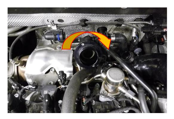
10. Push the Forge vacuum T over the vacuum port on the inlet manifold, secure it with the E-clip provided and reconnect the OEM vacuum hose (removed in Step 2.) to the other side of the Forge vacuum T.
