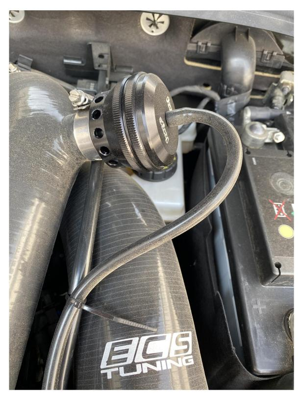
18. Connect the vacuum pipe supplied from the top of the dump to the boost take off adapter you fitted in section 14. Using the tie clips provided, fasten the vacuum tube to the coolant pipe pictured and arrowed white.
