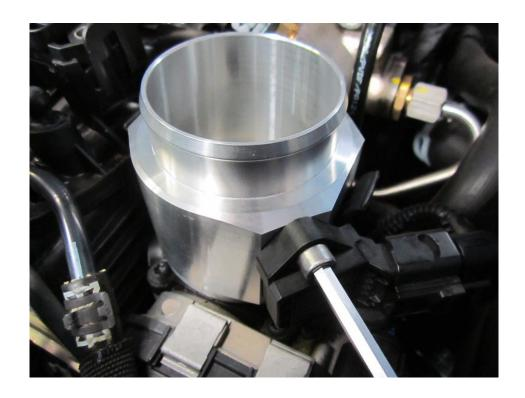
12. Remove the MAP sensor that is mounted on the inlet manifold. Again pry the clips apart while pulling on the sensor.
