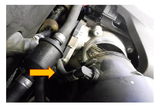
3. Disconnect the lower breather from the airbox by depressing the tabs on the Norma fitting as pictured below.
