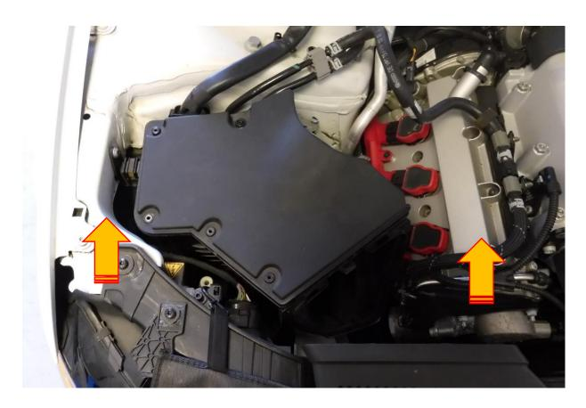
5. Remove the rubber grommets located on the underside of the airbox and locate into the chassis leg.
