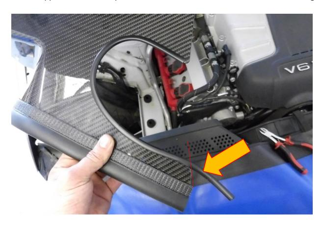
7. Using a 6mm Allen Key attach the fasteners to the carbon heat shield and supplied alloy pins.
