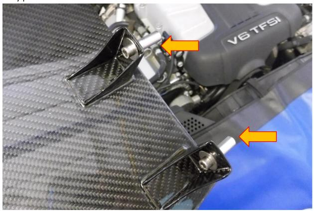
8. Mount the carbon heat shield into position ensuring the front of the carbon heat shield is located beneath the front scoop as pictured below.
