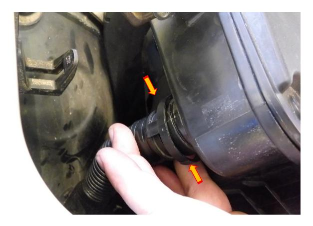
4. By pulling in an upwards motion remove the airbox from situ.
