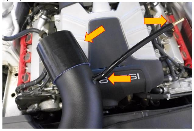
11. Attach the inlet pipe into position and connect the small brass connector to the hose removed in section 2, then place the filter onto the opposite end of the inlet pipe.
