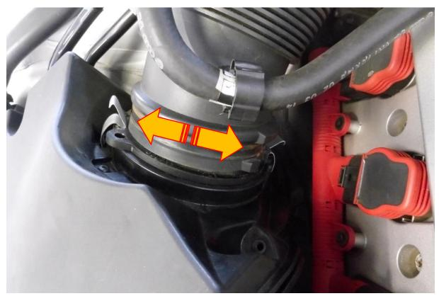
2. Disconnect the inlet tract at the throttle body and remove the vacuum hose pictured below.
