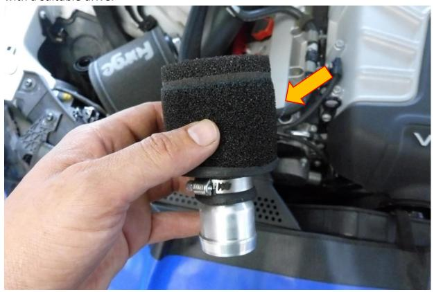
13. Fit the breather adaptor as pictured below and locate to the inner side of the wing.
