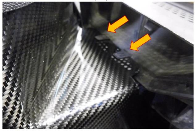
9. Using a 6mm Allen key tighten the fasteners fully as pictured below.
