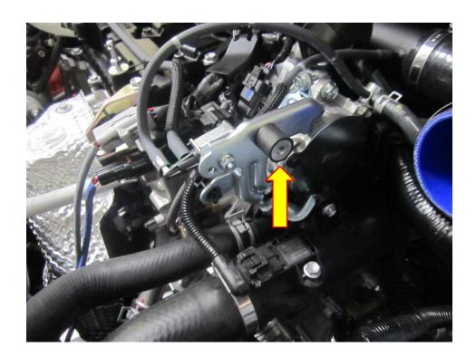
18. Attach the 90 degrees silicone hose with vac spout to the other end of the hard pipe. Make sure you have the hose clamp on the hose but loosely fitted. At the other end of the hose you can now fit the air filter. Do not tighten the hose clamp yet as you will need to adjust the filter position. The vac hose that went to the original air box fits to the vac spout on the new hose. Use the hose joiner supplied in the kit to attach them together.
