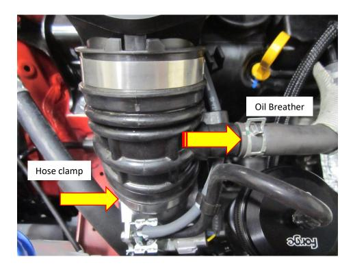
6. At this stage you can now remove the whole air box and pipe work as one. Lift the back of the air box to release it from its rubber mounting points. Make sure all the vacuum hoses are unattached from the intake pipe and you will be able to remove the air box. To do this, pull out the air box while twisting it 90 degrees to the left as shown in the picture.
