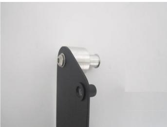
**11.** Once you have made up the mounting bracket, install it into the rubber lugs that held the back end of the airbox in place. The mounting bracket simply pushes into place.
