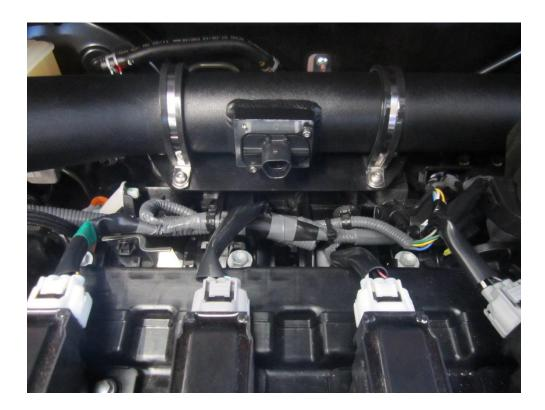
**14.** Plug the MAF sensor loom back into place and cable tie down the excess loom with the injector loom as shown in the picture below.
