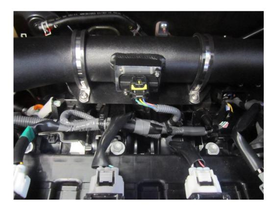
**15.** Fit the 90 degrees silicone hose with the oil breather spout. Loosely place the hose clamps around each end of the hose then attach the hose the hard pipe and the turbo elbow, then tighten the hose clamps with a 7mm socket and ratchet or a flat blade screwdriver. The oil breather will just push fit to the spout coming out of the silicone hose.
