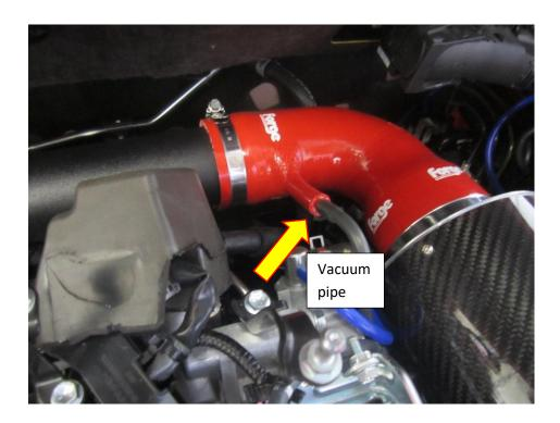
19. With the air filter now attached to the silicone hose and the Forge badge facing upwards, look inside the air filter and you will see a hole to the left side. Use a 5mm Allen key to attach the M6x8 bolt, M6 sprung washer and the M6 plain washer to the anti-vibration bush fitted earlier. This will keep the air filter firmly in place. You can now refit the alloy spinning back onto the air filter with the three Philips fasteners.
