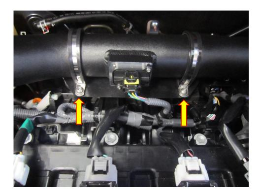
21. The final stage of the installation is to install the large silicone air intake pipe, the shorter end fits to the air filter and the longer leg of the hose locates under the near side head light through a gap in the wing. Once in position, tighten the hose clamp to secure the hose to the air filter. Now refit the engine cover by pushing it down into position. (The recommended torque setting is between 2 and 2.4NM please do NOT exceed this or the alloy spinning on the filter will deform).
