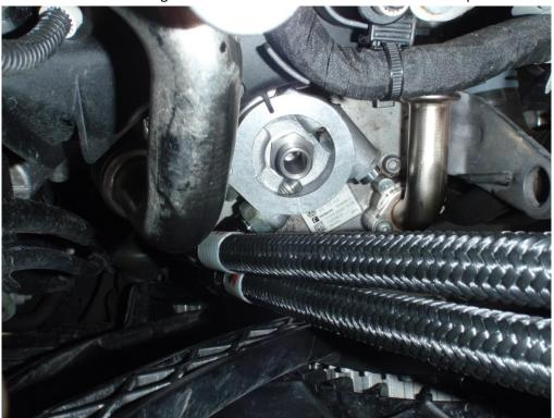
4. Feed the braded hoses through the radiator pack as shown below screw on the NA dash fittings and tighten. Please refer to the intercooler instructions to replace bumper.
