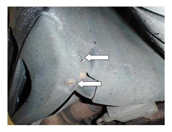
5. Working in each wheel arch undo the four T25 torx screws on the edge. Now remove the single T25 torx screw which goes vertically upwards into the rear wing.
