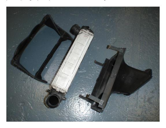
14. The new cores are slightly thicker so using a dremel or similar, you will need to remove plastic from both sides of the ducting as shown below, just leaving the vertical strips of plastic holding the clips on one side, and the clip receptacles on the other.
