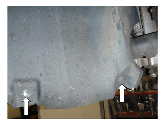
7. Now to fully release the bumper, remove the two torx screw either side of exhaust pipe on each side.
