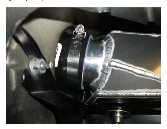
22. On the lower intercooler pipe, use the silicon hose supplied and secure with jubilee clips. The hose is subtlely different each side so they cannot be mixed up.
