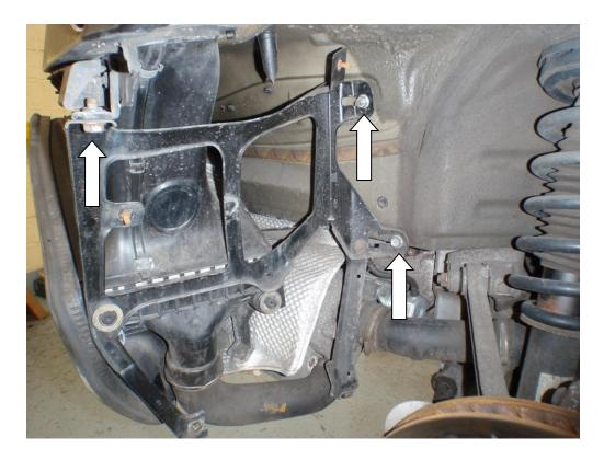
10. Now release the intercooler hose by inserting a screwdriver in the raised section of the clip and pulling it outward to release the hose. The other end is joined to the intercooler with a simple jubilee clip. Also undo the two 10mm screws holding the intercooler frame to the exhaust heat shield.
