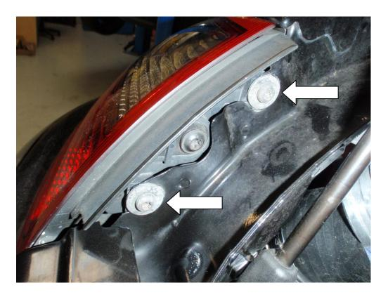
2. Remove the small plastic torx screw and pull out the plastic grommet.
