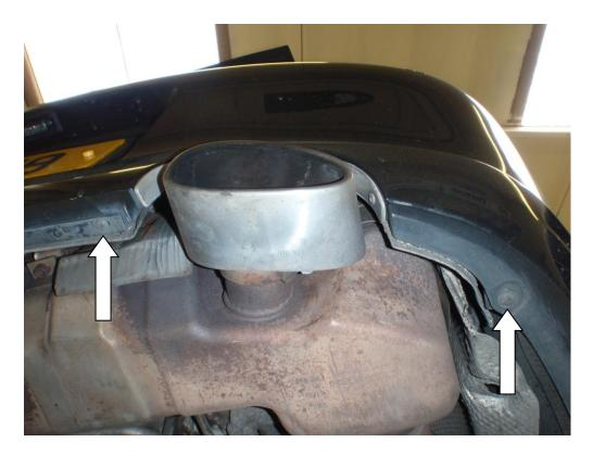
8. Now with the help of an assistant, tug the bumper rearwards off the plastic runners in the rear wings. When the bumper is pulled away enough, you will need to disconnect the electrical plug for the parking sensors and lights before removing the bumper completely and storing it somewhere safe.
