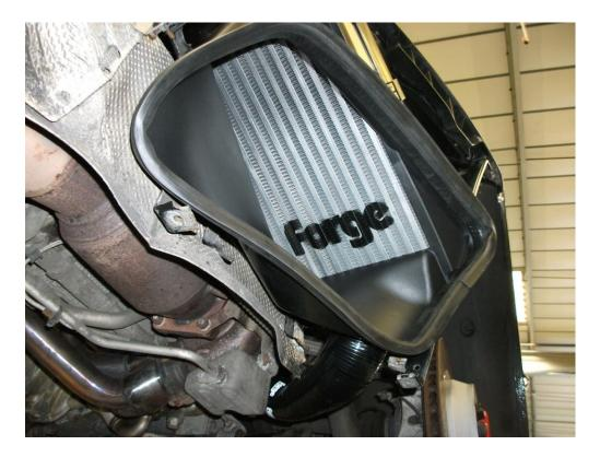
20. Position a jubilee clip over the end of the intercooler where it passes through the chassis and into the engine bay. You may need to completely undo the jubilee clip to pass it around the intercooler pipe.
