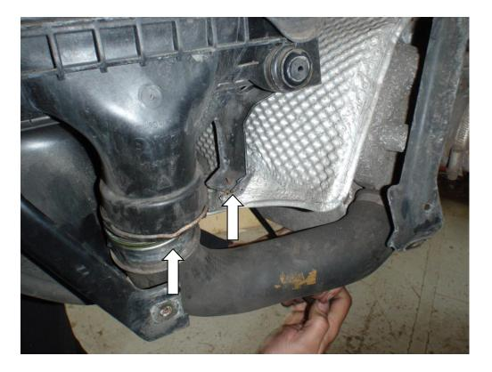
11. On the other end of the intercooler, remove the clip securing the intercooler outlet hose and pull it out into the engine compartment. The hose can now be removed from the engine. Remove the torx screw holding the frame to the exhaust heat shield, and the nut and bolt holding the frame to the car. The intercooler and frame can now be manipulated out of the car.
