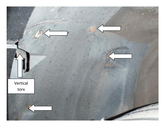
6. Finally remove the two torx screws at the bottom edge of the arch liner, then pull the arch liner off and remove from the car on each side.
