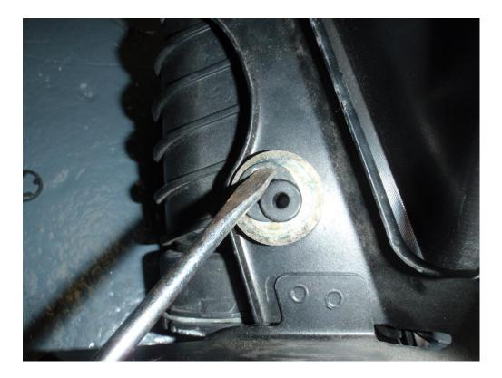
13. Unclip the upper and lower plastic ducting from the intercooler by pulling back on the end of the plastic clips – again you may need a screwdriver as these are tight.
