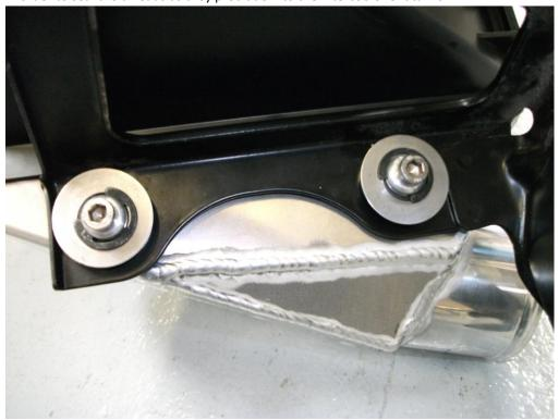
18. The bottom grommets are welded in position, use a pair of long nose pliers to reattach circlip.
