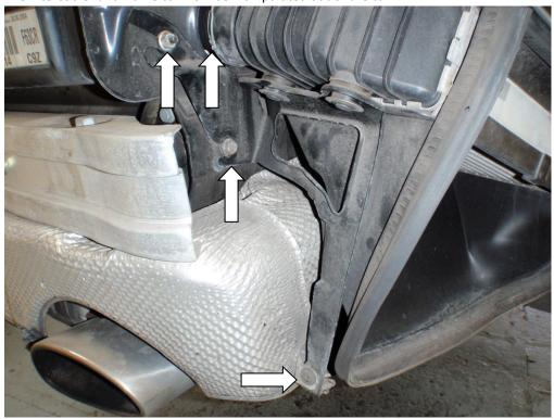
12. To remove the intercooler from the frame, prise the circlip out from each rubber mount, four in total. This will allow the grommet to be pushed through the frame and the intercooler with its plastic ducting to be removed. Retain the circlip and washers from each grommet for later use.
