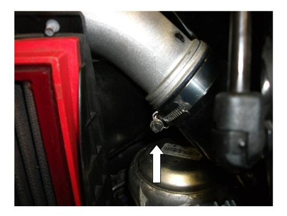
21. Position a jubilee clip over the end of the intercooler where it passes through the chassis and into the engine bay. You may need to completely undo the jubilee clip to pass it around the intercooler pipe. Tighten the jubilee clips.
