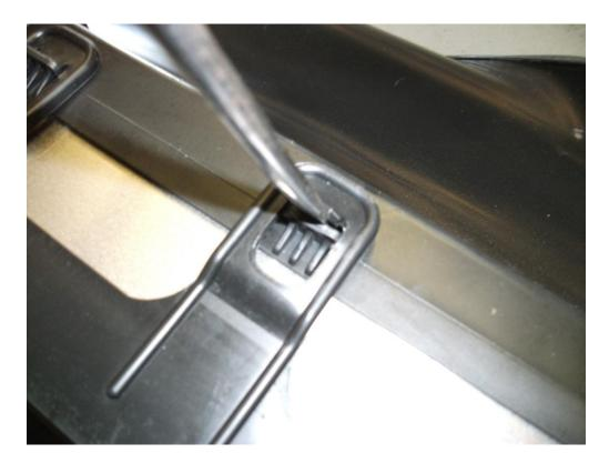
17. Push in the bottom end with the welded bosess, Line the threaded holes on the intercooler up with the rubber grommets on the frame. This time assembly is a little different – push the circlip onto the aluminium boss supplied FIRST, then place the washer under the circlip, then bolt the whole lot to the intercooler through the rubber grommet as shown below. You MUST use Loctite or a similar product in order to seal the threads as they protrude into the intercooler endtanks.
