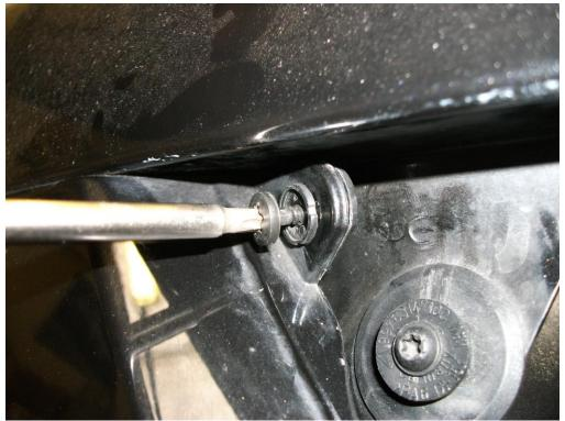
3. With both lights removed, undo the four torx screws that hold the top of the bumper
