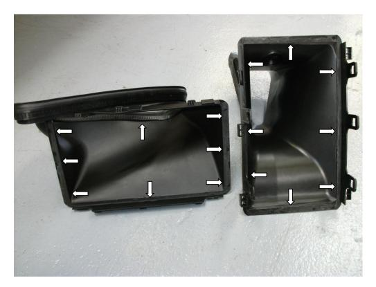
15. Of the two Forge intercoolers supplied, find the correct one for the side you are working on and reassemble it into the plastic ducting. Ensure that the ducting is offset to the core as you fasten all the clips.
