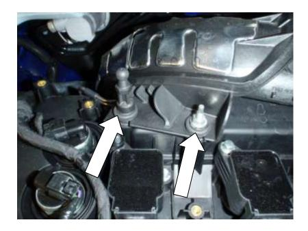
9. Using a hose clamp driver or similar tool undo the central jubilee clip.
