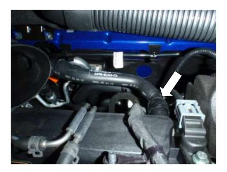
12. Using an 8mm socket undo the MAF sensor bolt and remove sensor from the standard air box.
