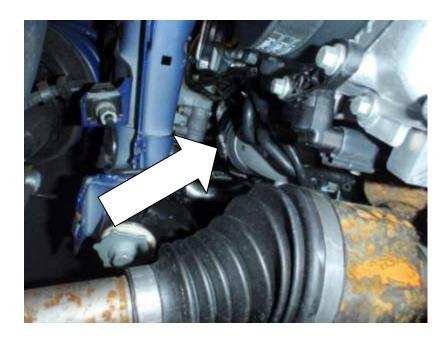
8. On top of the engine, using a 10mm and 12mm spanner undo the 2x fixings.
