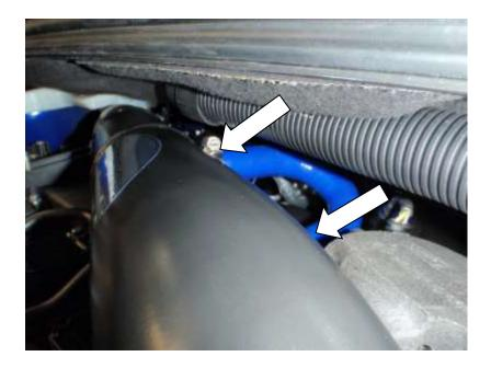
14. Place the 63/76mm silicone reducer on the turbo inlet and secure with a suitable JCS clip.
