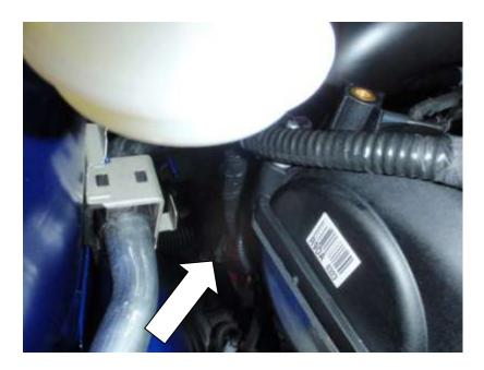
15. Place your Forge Induction pipe in position, connect the 19mm outlet to the open end of the silicone hose running from the cam cover, secure with a 25mm JCS clip. Bolt in place using the fixings provided.
