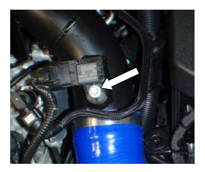
18. Using the 90deg. Silicone bend join the 76mm opening to the hard pipe and secure with the provided clip.
