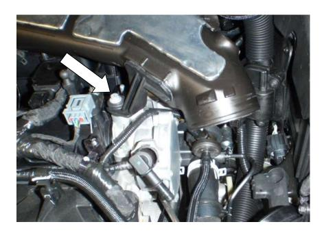
11. Unplug the standard engine breather pipe from the back of the cam cover.
