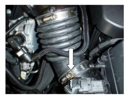
5. Unclip the the rubber cover that joins the air intake to the front of the car.
