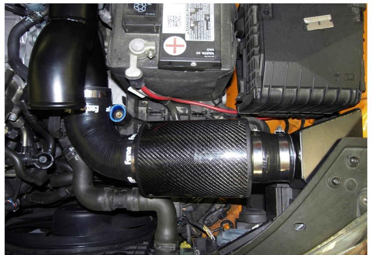
You will now attach the second carbon cannister using the remaining two 76-70 straight couplers. Due to the fixed nature of the pipe and the forward ram-air inlet duct, it will take some effort and manuevering to insert the cannister and attach both couplers to the piping. Once both couplers are attached to the piping, however, secure the hose clamps.
