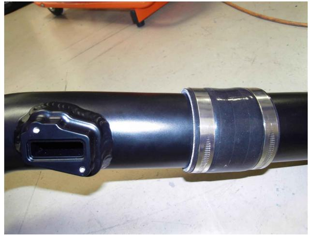
Now attach the piping assembly to the motor using a #70 hose clamp to attach the reducing coupler to the turbo inlet on the rear of the engine. If your vehicle is equipped with the noise pipe / engine amplification pipe, you may wish to remove this to give yourself more access to the hose clamps to attach the piping to the turbo inlet. Secure both hose clamps tightly.
