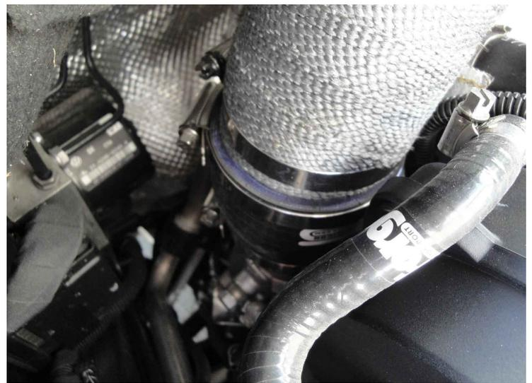
With the pipe now fitted to the engine, you will need to attach the two inlet ducts to the front end of the car. The forward facing ram-air duct will be attached to the front radiator support / slam panel using the original T25 Torx screws that secured the original intake ducting that were removed previously. The side duct is secured using the two T30 Torx screws that secure the upper edge of the radiator support just behind the headlight.
