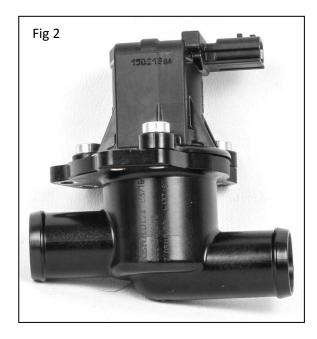
2. Remove the solenoid valve by undoing the 3 bolts using either a 4mm Allen key or T30 Torx driver.
