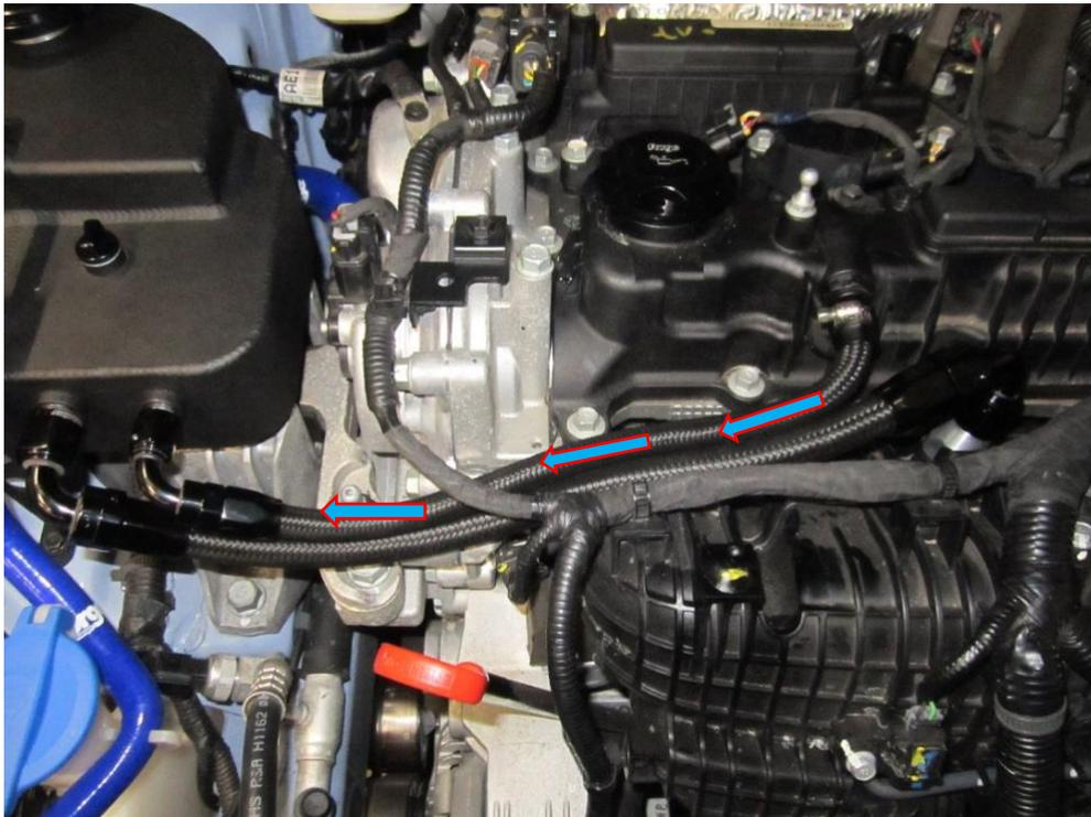
10. Take the longest hose from the kit and run the hose as shown in the picture below. Unclip the wiring loom to the injector behind the oil cap, this will allow you to run the hose underneath it, then re connect the loom. Use a 25mm spanner to tighten the AN-10 fitting and a 7mm socket for the hose clamp at the other end of the hose.
