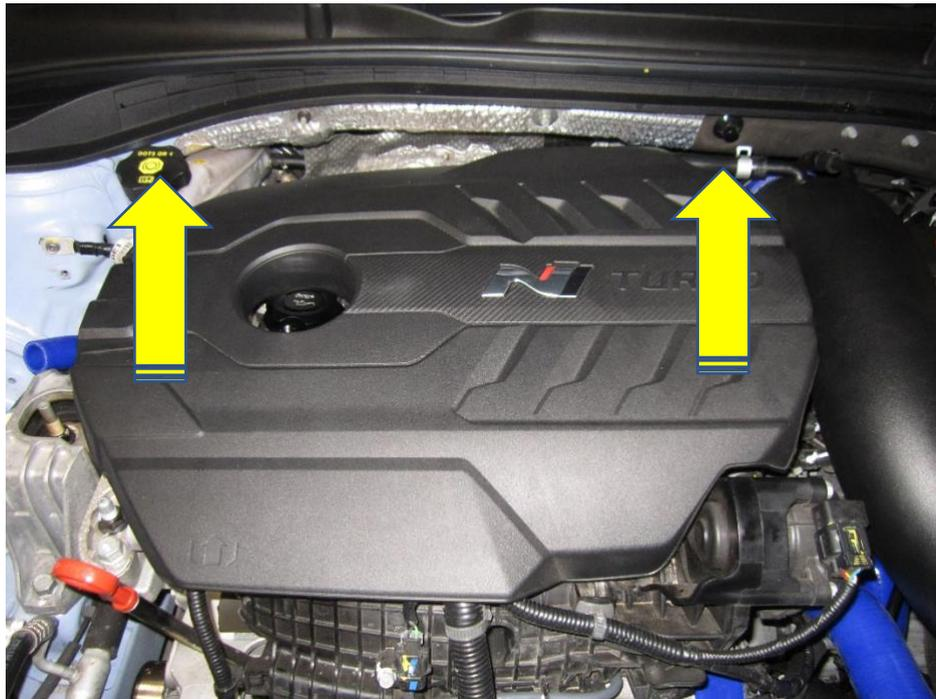
3. Locate the two breather hoses in the engine bay, the first one is at the front of the engine rocker cover and the second one is located at the back of the engine attached to the air intake pipe. To remove them release all four hose clamps in the same way as step one.
