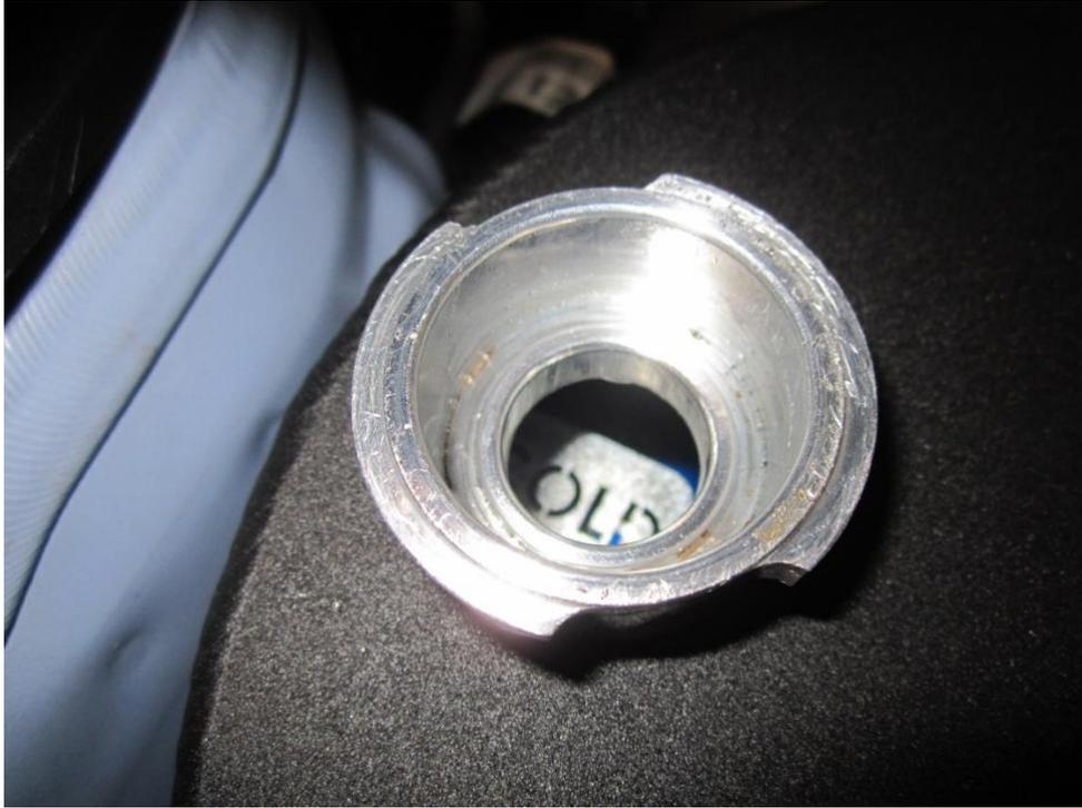
13. Take your original coolant cap and screw onto the Forge expansion tank. Once fully tightened place the Forge alloy cap over the OE cap line it up and fix into position with the grub screw.
