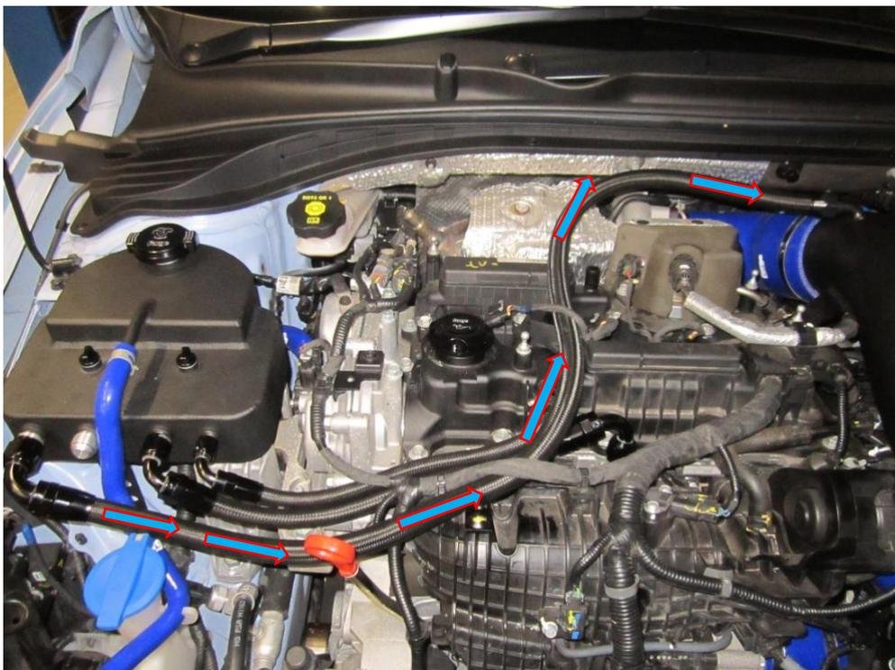
11. The last hose to be installed is another AN-10, run the hose as shown in the picture. The breather end is another push fit.
