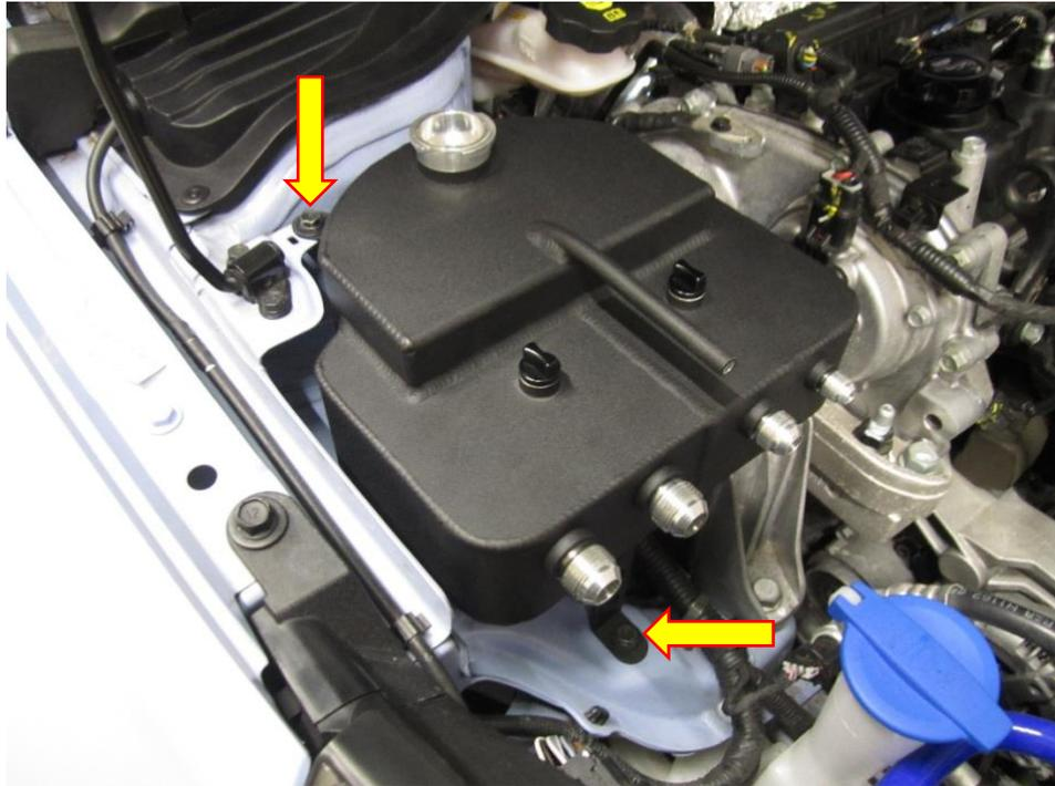
6. From the FMCT5 kit, take the two rubber grommets and two alloy fittings. Make sure that the plane rubber grommet is inserted into the short fitting and the ribbed rubber grommet is fitted to the taller alloy fitting. Now fit each fitting to the appropriate 120 degrees dash fitting from two of the braided hoses from the kit. They can only fit one hose as they are different thread sizes. Use a 26mm spanner and an adjustable spanner to tighten.
