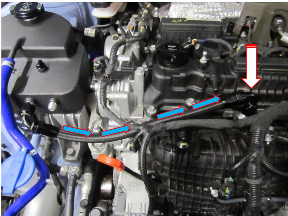
9. Attach the AN-6 fitting of the smaller hose to the catch tank and run the hose to the rocker cover as shown in the picture below. Use a 17mm spanner to tighten the AN-8 fitting and a 7mm socket to tighten the hose clamp on the breather end of the hose.
