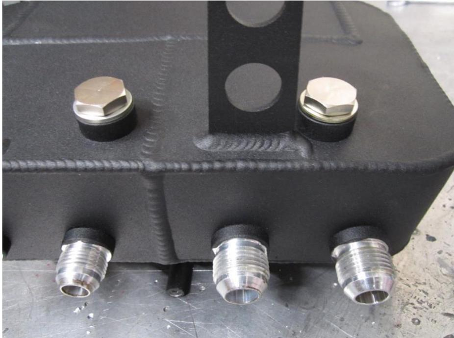
5. Fit the FMCT5 into the same location as the OE expansion tank, fit the lower coolant pipe using the original hose clamp. Secure the tank into place with the fasteners used to hold the OE tank as shown in the picture below
