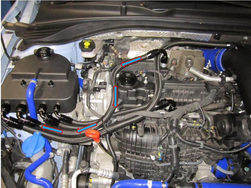
12. Re fill your coolant into the expansion tank, there is a maximum level indicator, the coolant should be just below this indicator. You may need to top this up after a few miles due to the system still bleeding any trapped air.
