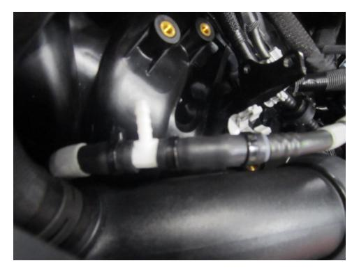
6. There is a 10mm fastener located above the dip stick, move the plastic hose above it to gain access to the fastener. Use a 10mm socket and rachet with an extension and remove the fastener.
