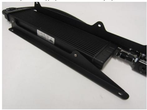
26. Using your m10 socket or spanner attach the oil cooler assembly to the condenser and radiator where you removed the fasteners in section 11.
