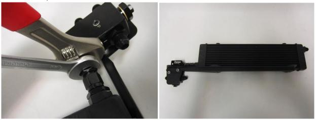
24. Attach the an-8 hose fitting to the oil cooler assembly again making sure you hold the hex on the opposite fitting to which you are tightening.
