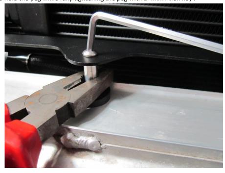
34. Tighten all your fasteners and bolt your crash bar fully into position.
