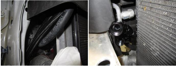
$18. \ Place the crash bar back in situ using only one fastener either side the tighten both them both fully .\\$
