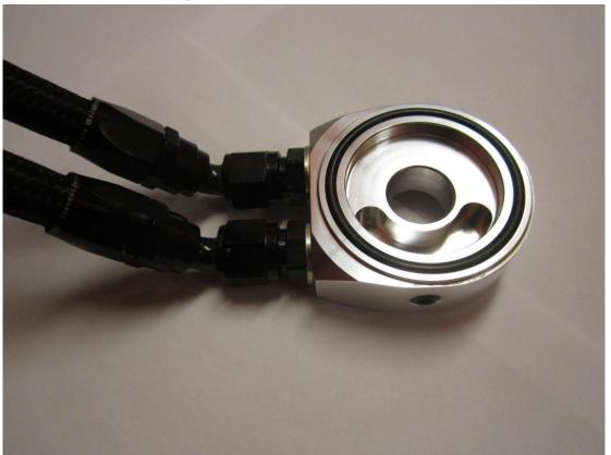
17. Clean the sealing face for the oil filter, a small amount of clean oil should be smeared on the sandwich plate along with the oil filter when being installed. Follow the next 3 pictures to ensure you place the oil lines in the correct position then mount the sandwich plate into position with the oil cooler extender bolt, this only needs to be finger tight at this moment.
