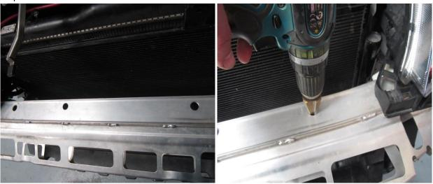
29. Insert the 3 rubber grommets into the holes you have drilled in the crash bar.
