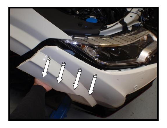
5. With the sides of the bumper pulled out unclip the spot lights on both sides and parking sensors.
