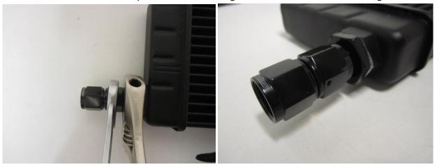
22. Hand tighten the remote oil thermostat housing onto the female fitting and place the spacers in place ready to fit the lower frame assembly to the oil cooler.
