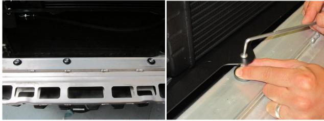
33. Once these have been finger tightened in the correct location slide the crash bar downwards then use a pair of pliers to hold the peg while fully tightening the peg with a 4mm Allen key .
