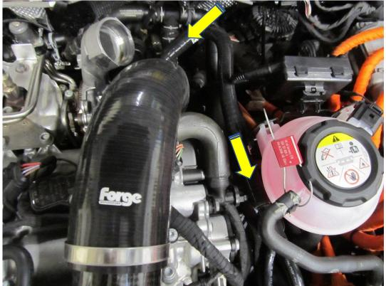
**14.** Use silicone spray in the end of the turbo inlet pipe to help when fitting the airbox into situ not forgetting to connect the engine breather to the airbox.
