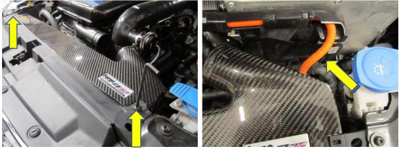
**16.** Fit the OEM flexi pipe from the carbon duct to the carbon airbox.
