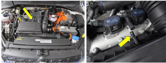
4. Remove the hose clamp that holds the airbox to the turbo inlet hose.
