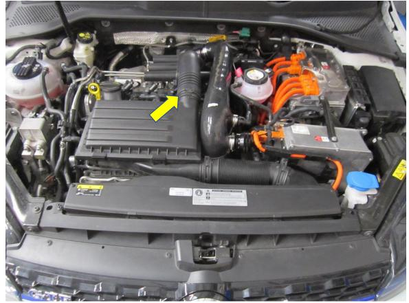
5. Remove the front air scoop and remove the airbox by pulling it sharply in an upwards motion.
