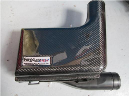
**13.** Fit the large bore high flow turbo intake into position but do not tighten the hose clamps. Fit the breather hose to the outlet spout and the other end to the OE breather hose.
