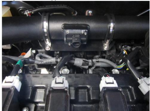
14. Now you can plug the MAF sensor loom back into place and cable tie down the excess loom with the injector loom as shown in the picture below.
