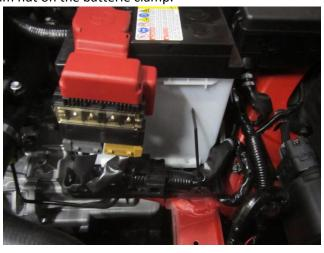
9. With the terminal tightened up, you can now tidy the wiring loom, first tuck the excess loom round the back of the batterie and cable tie it to the loom coming from the fuse box. Now working backwards cable tie the next part of the loom using the existing fastener hole.
