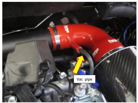
19. With the air filter now attached to the silicone hose and the forge badge facing upwards, look inside the air filter and you will see a hole to the left side. Use a 5mm Allen key to attach the M6x8, M6 sprung washer and the M6 plane washer to the rubber cotton reel fitted earlier. This will keep the air filter firmly in place, you can now re fit the alloy spinning back onto the air filter with the three Philips fasteners.
