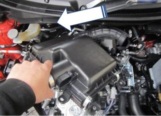
7. Before you can install the FMINDK29 you will have to re locate the positive side wiring loom to the vehicle batterie. There are four plastic fasteners the need to be undone use a flat blade screw driver to prise the clip off. At this stage disconnect the NEGATIVE Batterie terminal with a 10mm spanner/socket & rachet.
