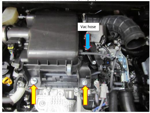
4. The MAF sensor will now need to be removed, first unplug the sensor then remove the two Philips screws locating it in place with the use of a Philips screw driver. Now carefully remove the sensor from the air box. Un clip the MAF wiring harness
