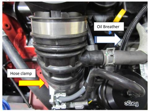
6. At this stage you can now remove the whole air box and pipe work as one, lift the back of the air box to release it from its rubber mounting points. Make sure all the vac hoses a un attached from the intake pipe and you will be able to remove the air box. To do this pull out the air box while twisting it 90 degrees to the left as shown in the picture.
