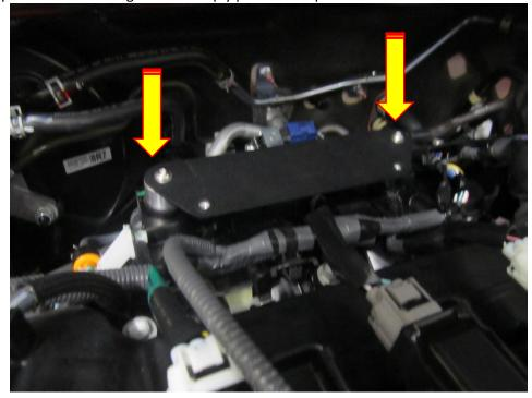
12. Take the hard pipe from the kit and mount the original MAF sensor into the MAF boss on the hard pipe, there are two m4 fasteners with kit with the use of a 4mm Allen key tighten the sensor to the MAF boss.
