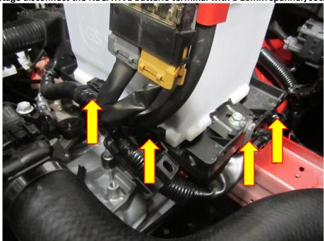
8. Slacken off the 10mm nut on the POSITIVE batterie clamp so that you can twist it 90 degrees to the right. Pull the wiring loom round so the you can move the batterie terminal into position, when you have got the terminal into the desired position tighten the 10mm nut on the batterie clamp.
