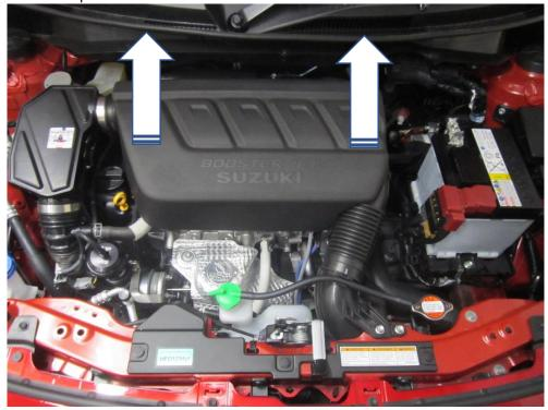
2. The air scoop/intake at the front of the engine bay is held down with four 10mm fasteners these need to be removed with a 10mm socket and drive. You can now remove the air scoop and hose (all three parts) from the engine bay.
