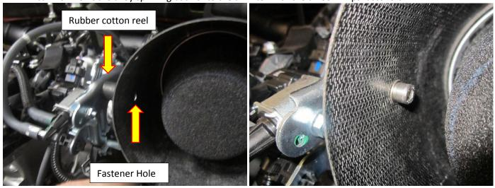
20. Now with the filter in place go back to the mounting bracket and tighten the M6 fasteners and all the hose clamps for the silicone hoses.
