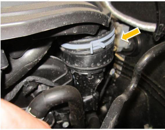
5. Using a T25 Torx Drive remove the fasteners that hold the front air duct in place.
