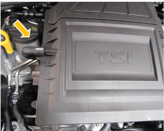
3. Using a T30 Torx Drive undo the fastener that holds the airbox in position.
