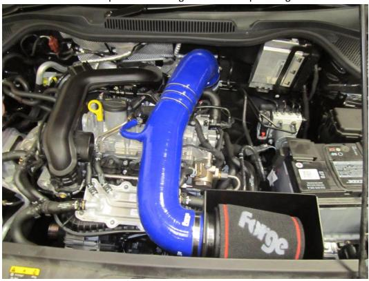
**13**. Remove the OEM breather hose and attach the new hose, do not over tighten the hose clamp as this could break the plastic OEM breather fitting.
