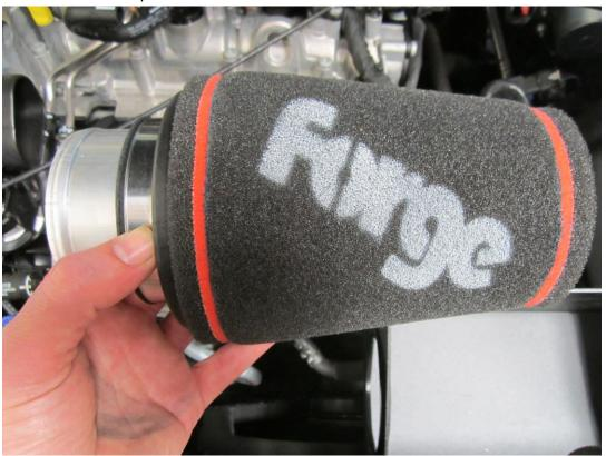
11. Now fit the Forge Motorsport Airfilter into the air intake tray, a small amount of silicon spray will ease the fitment of the filter coupler through the air intake tray hole.
