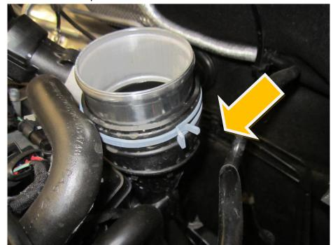
9. Fix the air intake tray into position using the OEM fasteners with the T25 Torx Drive.
