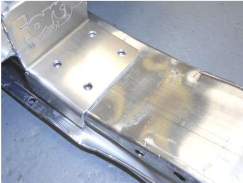
53. Using a drill and 5mm drill bit drill the 8x holes.
