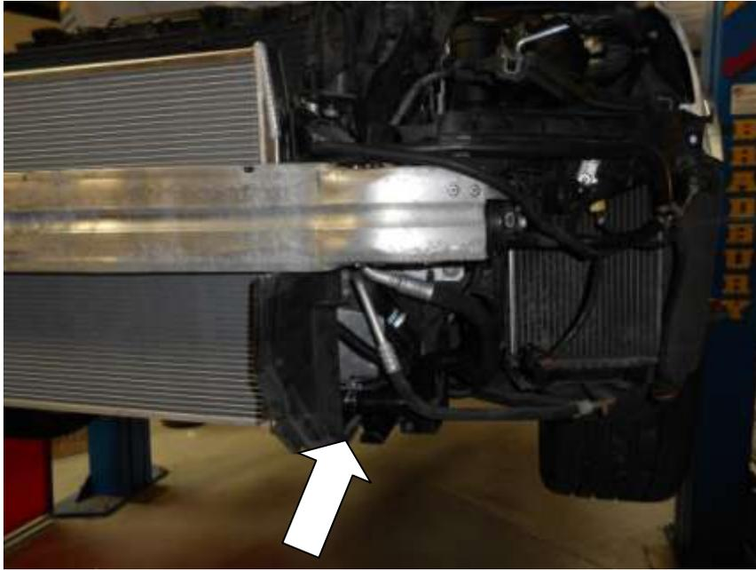
61. Refit the secondary radiator and fit **F** and **G** silicone hoses to the correct outlets and secure with suitable hose clamps.
