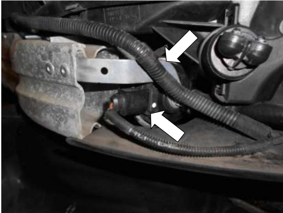
17. Unclip the secondary radiator ducting and remove it from the vehicle.
