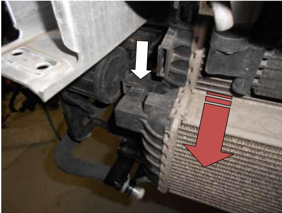
24. To allow better access to the pump and secondary radiator. Undo T30 screw and unclip hose clips.
