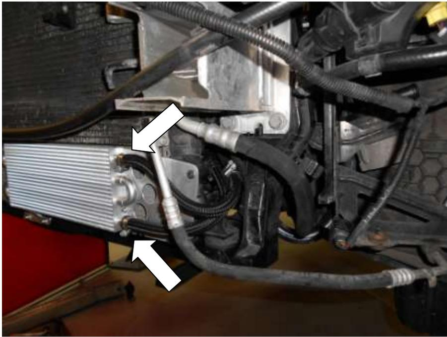
45. Cable tie rubber pipes to back of the fan shroud. Make sure the fan can still rotate freely.
