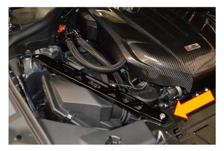
2. Located in the inner wheel arch where the strut mounts to the body, you will see the 8mm Allen Cap protruding through the strut top. Place the washer and Nyloc nut on the bottom of the fastener. Using a 10mm socket and suitable drive, hold the nut in position and tighten the Allen Cap using a 6mm Allen key from above.
