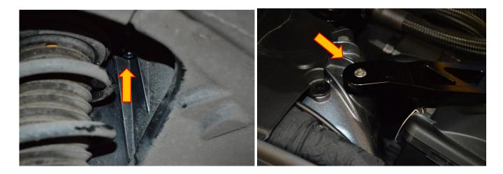
3. The M10 Fastener may now be torqued to 42NM and the M8 Fastener may be torqued to 20NM.
