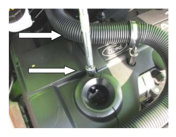
Remove the two T25 Torx bolts from the cam belt cover. And slide the cover off.
