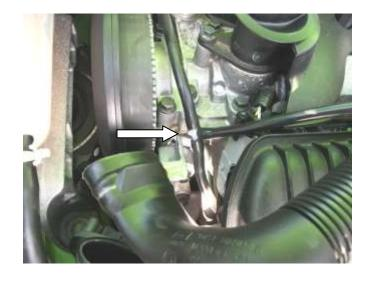
Cut the original rubber vacuum hose in the shown location
