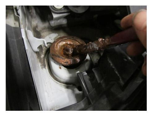
9. You can now attach the FMSTC1's to your vehicle. Make sure you have them lined up and slowly screw them on in a clockwise motion. If it feels quite stiff to turn at any point undo them and check the thread on the shock absorber for damage or dirt.
