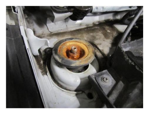
7. Use a wire brush to clean the thread on the vehicles shock absorber, make sure it's totally free of rust and dirt. Blow out excess deposits so the area is as clean as possible.
