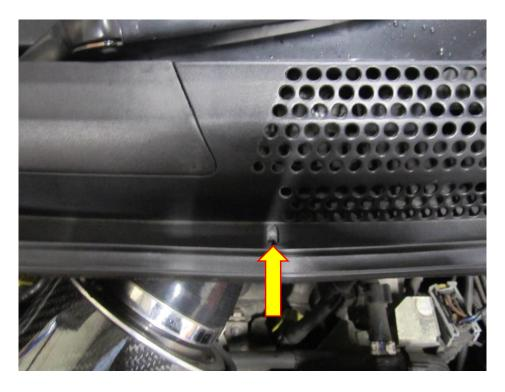
2. Remove the rubber weather strip located at the bottom of the scuttle panel. This just pulls off with gentle force.
