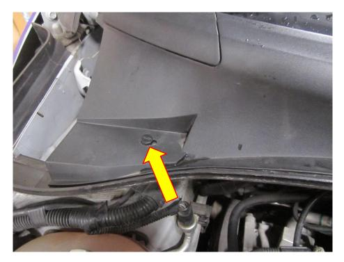
4. There are two covers that obscure the wiper spindles which need to be removed. These covers just pull away to release them.
