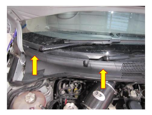
5. Using a 13mm socket and ratchet remove the fasteners holding the wipers in place. With the fasteners removed you will now be able to wriggle the wipers free. The scuttle panel can now be removed from the car, just remember to disconnect the water washers.
