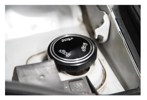
10. With both FMSTC1's fitted you can now put the vehicle back together in reverse order to dismantling it. Just one tip to point out is making sure the clips of the scuttle panel go under side of the windscreen.
