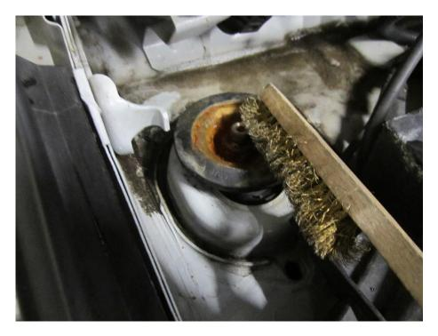
8. Lubricate the whole of the strut top especially rubber cover.
