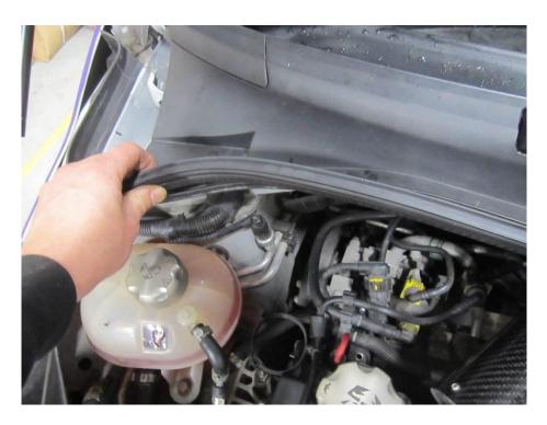
3. Next, remove the two plastic fasteners each side of the scuttle panel. Use a flat blade screwdriver or trim tool to do this.
