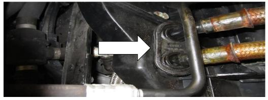
17. The fan controller can also be removed now. Undo the three wiring harnesses then remove the 10mm nuts holding on the control unit.
