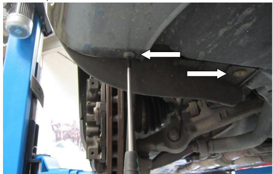
4. Inside the wheel arch undo the T25 fasteners pictured.
