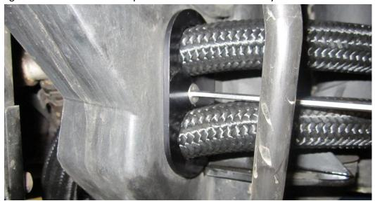
34. Place the oil hose clamp in position and tighten.
