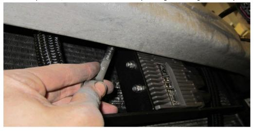
30. Now fix the upper two cotton reels on the power steering cooler to the lower part of the oil cooler bracket using the existing m6 nuts that were removed in section 13
