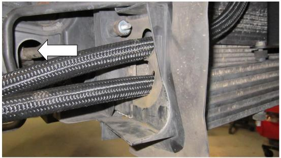
32. Connect the oil lines to the sandwich plate and tighten.
