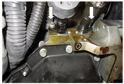
13. Next to remove the oil cooler undo the 10mm nuts in these locations.
