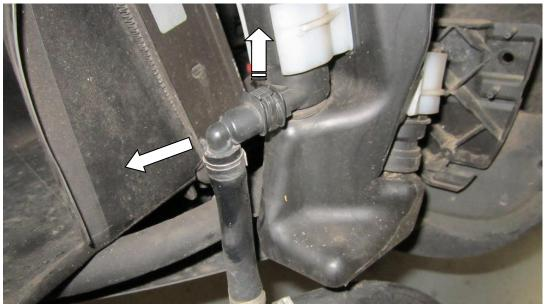
12. You are now ready to remove the OEM oil cooler. Start by removing the oil lines from the engine block. Use a T30 torx drive, have a drip tray or similar to catch the excess oil which WILL drip out of the block and old oil lines. Please make sure you dispose of the oil responsibly!
