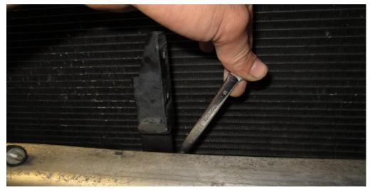
19. Now the fan control unit has been removed, place it onto the new Forge Motorsport bracket, using a 10mm spanner to tighten the 10mm nuts.
