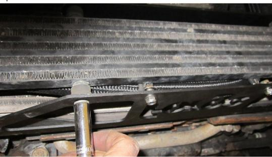
40. Place the two nylon blocks on top of the oil cooler and slide them over the condenser.
