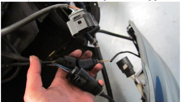
11. You also need to disconnect the washer jets, by pulling up the retainer and pulling out the hose. Have a jug ready to collect any screen wash you wish to keep.
