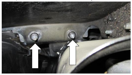
7. Moving to the front on the bumper remove these fasteners arrowed with a T30 torx drive.
