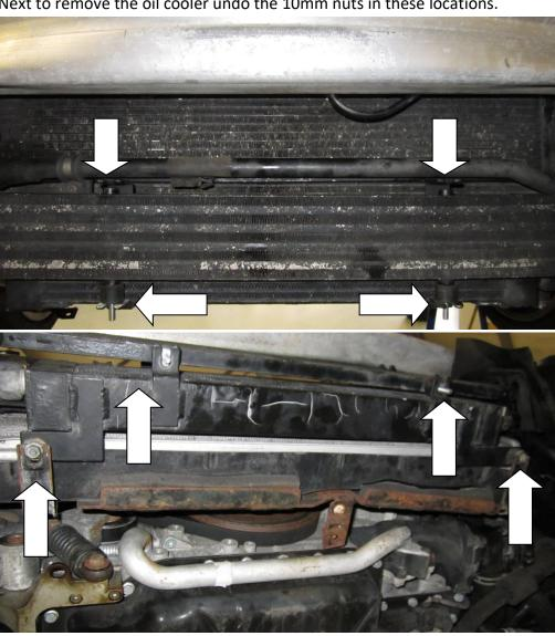
14. There are two final 10mm nuts tucked away behind the plastic cowl to remove. The other 10mm can be found in the same place but on the opposite side.
