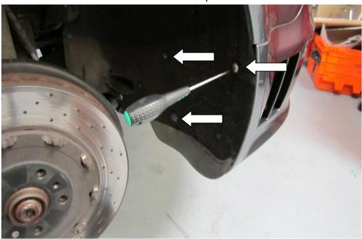
5. Pull back the arch liner, and behind you will find two more T25 torx fasteners. Remove these also.
