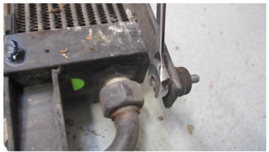
37. Place the lower Forge mounting bracket into position. Use the cotton reels just removed to attach at the back of the mounting plate. Please note the orientation of the plate as this is handed i.e. its offset to one side.
