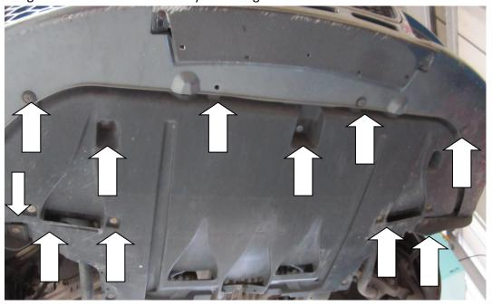
3. Using a T30 torx driver, undo the fasteners pictured. They are towards the rear of the under tray in the corners.
