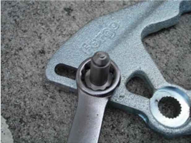
For the side-to-side linkage, the procedure is the same. You will need to select the cable shaft that matches your OEM linkage and attach it using the supplied 13mm lock nut. Position the shaft at your desired adjustment location and tighten it securely in that position.
