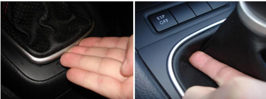
Position the shift lever so that the two alignment holes allow you to position the included nail into the holes as show below thus locking the lever in place.
