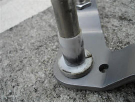
Reinstall the replacement front-to-back linkage by sliding it onto the splined selector shaft. There is a singular large locator spline that will only allow you to install the linkage in only one position. It may take some maneuvering to find this locator spline and slide the linkage onto it, but it is not difficult.
