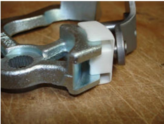
Once both linkage components are reinstalled and the “E” shaped guide is positioned properly, insert the second white plastic center shaft bushing into the pivot mount as shown below.
