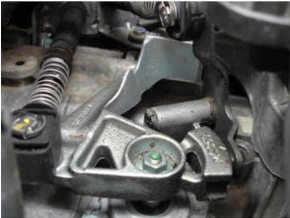
Once you have gained access to the shift linkage, begin by removing the two circular clips securing the black plastic cable ends to the linkage.
