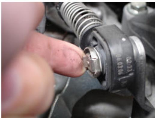
Also remove the small circular clip from the center pivot of the side-to-side linkage component.
