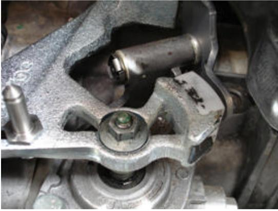
The linkage will twist clockwise when retightening this 13mm nut, thus engaging 3rd gear, so please return this linkage to its "neutral" position. In its neutral position, you will be able to freely push the linkage up and down into the transmission casing with very gentle effort. DO NOT reattach the black plastic cable ends yet as they still need to be adjusted.
