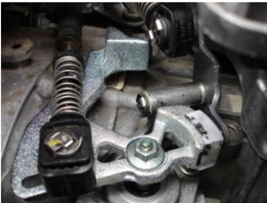
Keeping the actual shift linkage in its locked or neutral position, loosen BOTH black plastic cable ends by pulling the knurled ring against the spring tension towards the end of the cable and twisting it which will lock it into its "open" position.
