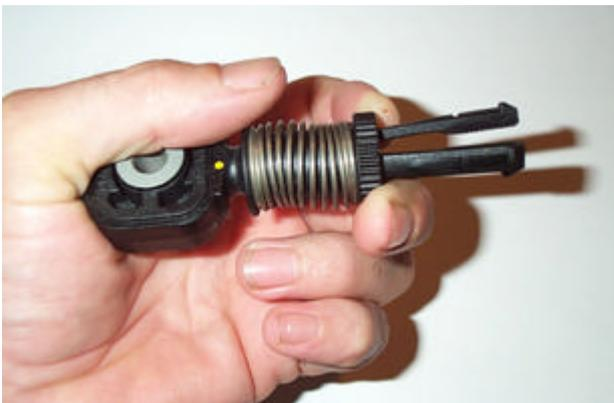
This loosening process alone should release any tension on the shift cables from misalignment due to the new shorter throw of the new linkage components.
