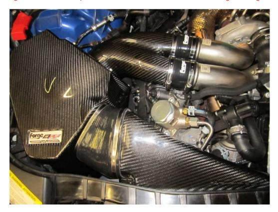
18. Once the intake has been fully fitted use the forge polishing cloth and meguiars gold class polish to remove any grease marks or finger prints from the carbon fibre .
