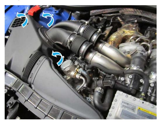
9. Using a 4mm allen key ensure the 4 allen caps that hold the performance airfilter into the carbon fibre airbox are tight.
