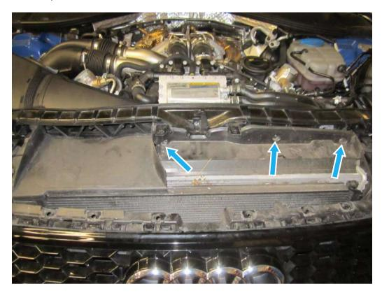
6. Using a T30 torx drive, remove the two fasteners that hold the cold air duct to the airbox, the duct will then be able to be removed from situ.
