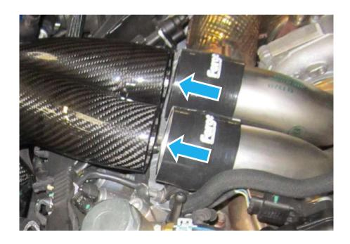
16. Now attach the cold air scoop to the carbon fibre front duct by using the T30 torx drive and fasteners.
