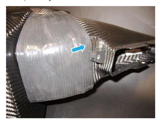
Alternatively the scoop can be attached to the airbox prior to installing the complete airbox into the oem rubber grommets, again with this method do not tighten any of the hose clamps yet.
