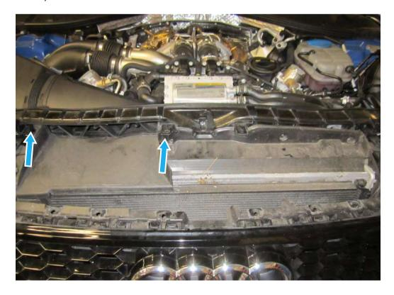
7. Using your 7mm hose clamp undo the two outlet hoses from the airbox that feed the inlets to the turbos .
