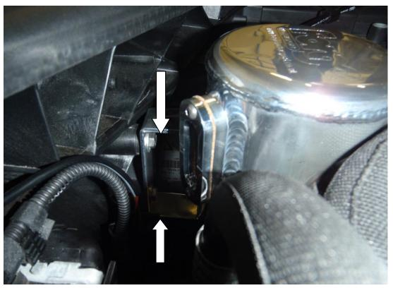
Now using the silicon hose provided cut it to desired length and fit each outlet on both the catch tank and inlet plate, using the 4 jubilee clips provided and tighten with a 7mm hose clamp driver.
