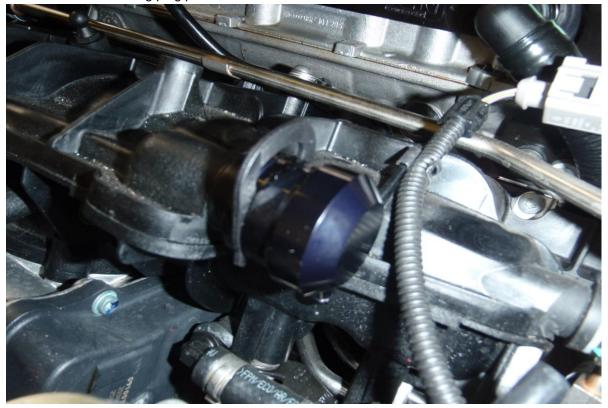
Next, **very carefully** use a flathead screwdriver to unclip the connector on the extreme right end of the PCV assembly.
