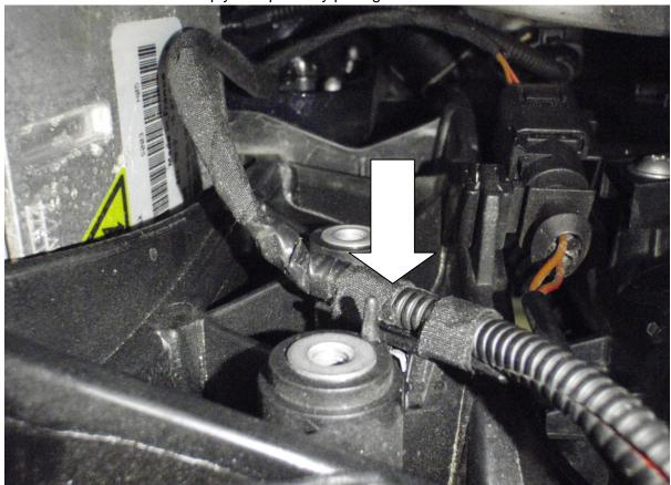
Fit the new catch tank into the threaded holes situated on the radiator cowling, using the two 10mm bolts provided as seen below.
