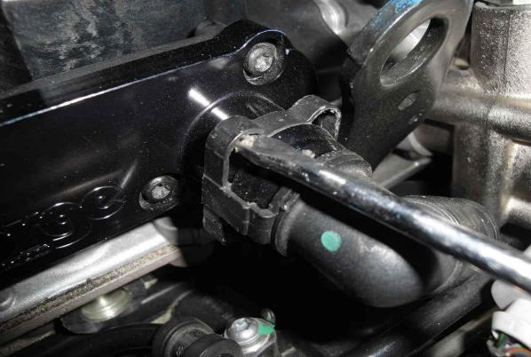
Next, using the T25 Torx bit, remove the 4 screws securing the PCV assembly to the valve cover. Save these screws as they will be re-used.
