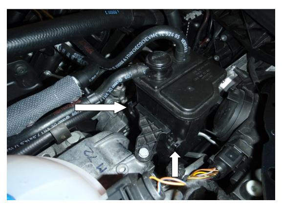
Before fitment of the catch tank you will see there is a wire running through where the bracket needs to bolt to. Simply unclip this by pulling it off.
