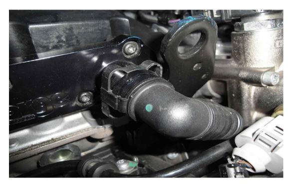
Before the fitment of the catch tank can take place you will have to unclip the charcoal canister by pulling upwards and just move it to the side just enough to make it easier to fit the catch tank.
