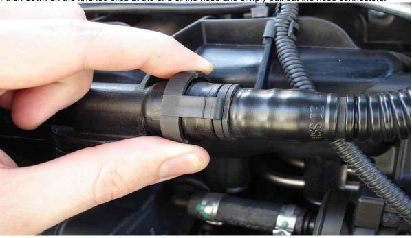
Fit the new inlet blanking plug provided to inlet manifold.
