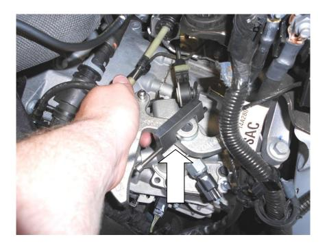
10. Using a 16mm spanner tighten the adjustable ball and locking nut supplied in the required position on the Forge Quickshifter. Closer to the pivot will give a shorter shift and further away will give a longer shift. To start with set the adjuster at the midway position.
