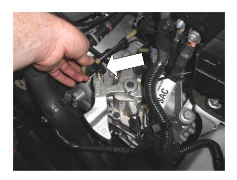
8. Place the Forge pin removal tool in position and using 5mm Allen key tighten to remove the locking pin.
