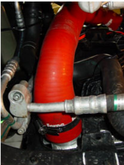
The new hose can now be installed and the lower hose clamp fitted and tightened.
