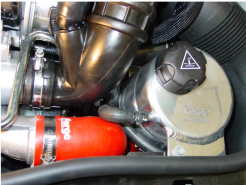
The Coolant Header or Expansion tank can be refitted.
