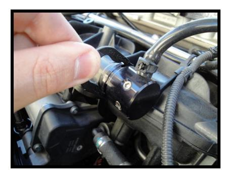
4. Attach the inlet manifold blanking kit with the plastic clip and screw in the appropriate grub screws or boost gauge ports according to your needs.
