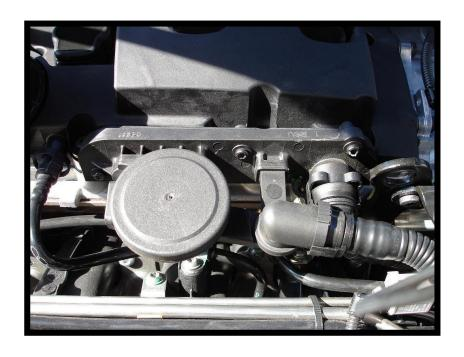
1. Unclip the breather pipes and undo the torx bolts, remove the PCV but keep to one side the rubber seal and torx bolts.
