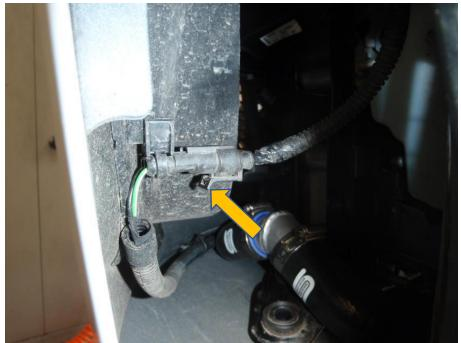
3. Looking under the car up at the arch liner there is a pozi drive/Phillips screw, undo this on both sides of the vehicle.
