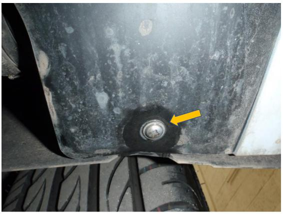
4. Undo the six bolts on the under tray using a 10mm socket and ratchet and remove.
