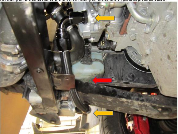
15. The longer AN-10 line is fitted from the top of the cooler to the top of the sandwich plate. Feed the AN line between the chassis leg and washer bottle as arrowed above in red. Please also study the following pictures below for the correct oil line routing.
