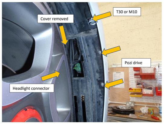
2. Additionally on the left-hand side you will need to pull back the arch liner. You should see another connecter (see below). Pull the clip down and pull away to disconnect.
