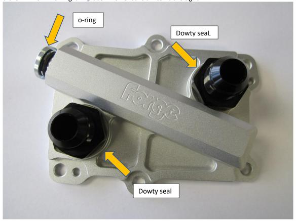
13. Remove the OEM sandwich plate from situ using a T30 Torx Drive to remove the 6 fasteners, you will need to have a suitable container to catch the oil and water once the sandwich plate is removed. Then fit the Forge Motorsport sandwich plate into position ensuring the factory seals are in place.
