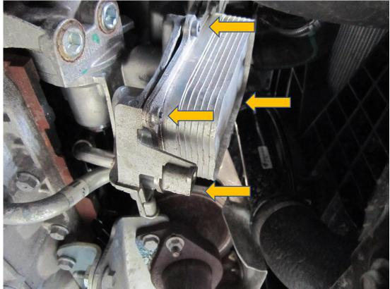
14. Now the sandwich plate is installed, fit the two AN-10 lines - the shorter line goes from the lower AN fitting on the oil cooler to the lower AN fitting on the sandwich plate as pictured below.
