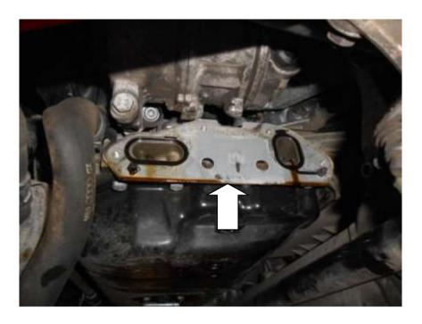
7. Using brake cleaner or similar clean any debris or oil from the mating surface.
