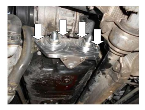
11. Bolt the brace plate in position with the remaining 2x M6x16mm bolts and reuse the OEM bolt for the sump fixing point.
