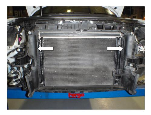
13. Undo the T30 torx and T25 torx holding the intercooler to the radiator pack and chassis. The red arrows indicate where four T20 screws are positioned behind the crash bar support.
