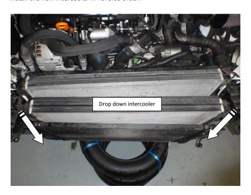
17. Attach the new intercooler with the bolts supplied in kit. The longer bolts attach the airconditioning to the intercooler, See step 18. The shorter bolts are for the radiator fitting to the intercooler.
