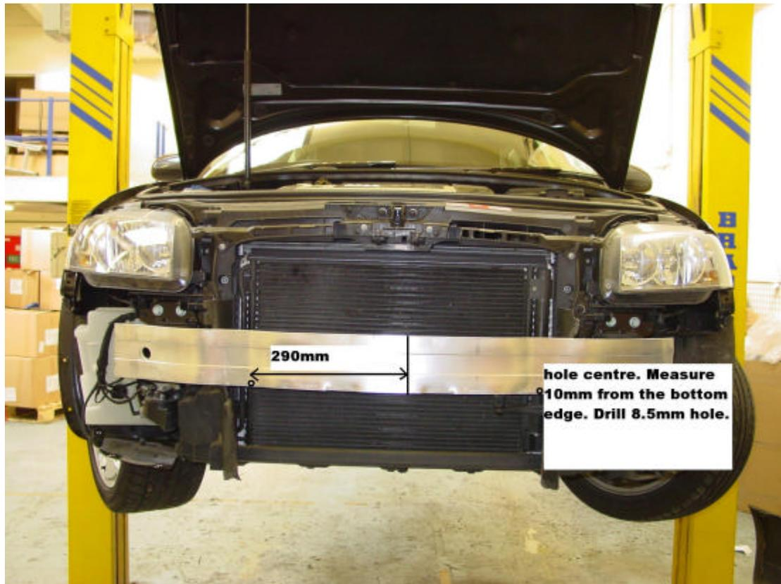
Fit the supplied brackets to the crash bar with the nuts & bolts supplied. Fit the intercooler to these brackets as shown. Tighten all the brackets and intercooler fixings once the intercooler is positioned centrally.
