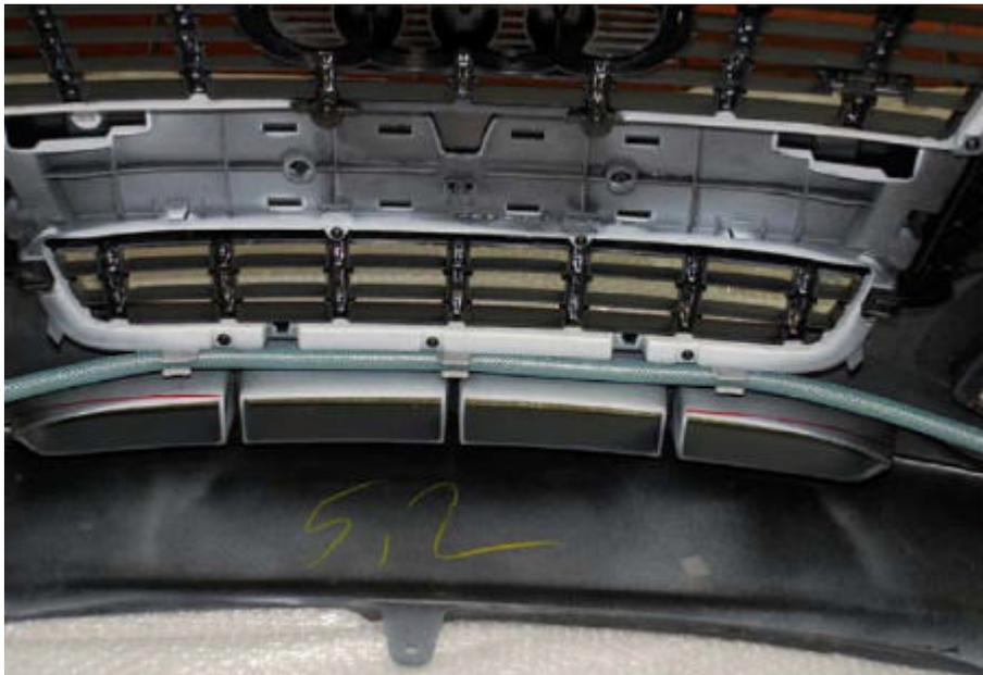
Again remove with a jig saw or open saw blade on both sides. Once the front panel has been trimmed refit it to the vehicle. If necessary trim more from any areas as required.
