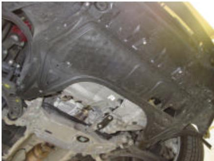
3/ Remove the 8x T25 screws in order to remove the complete engine under tray.
