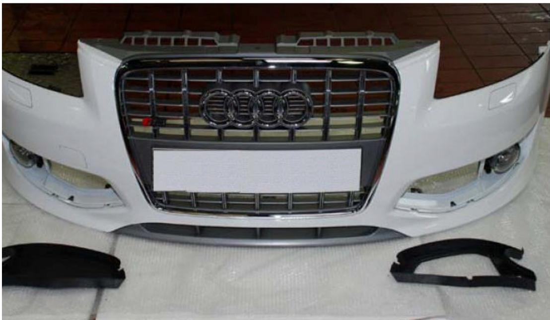
The lower grills need to be removed from the front panel on both sides. Then the grill backing panels are removed, these will not be refitted.
