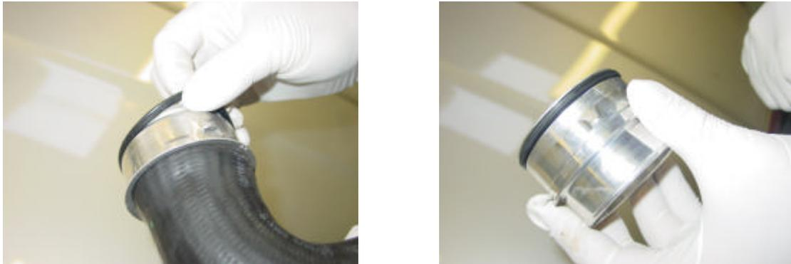
The new hose is fitted to the OEM intercooler with the hose clamps supplied.
