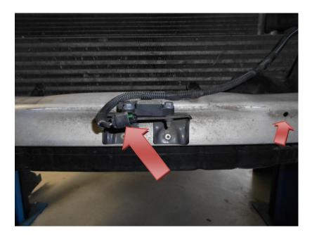
13. Using a 13mm spanner and an E10 Torxs socket undo the bolt at each end of the crash bar and remove it.
