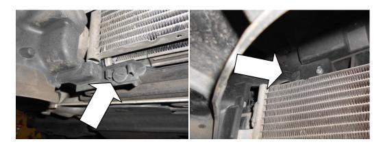
15. Using an 8mm socket undo the clips on the standard hose running to both sides of the intercooler.
