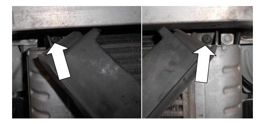
17. Slide your New Forge intercooler onto the original bottom intercooler mounts.
