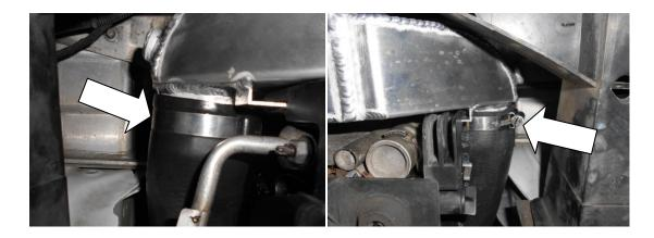
20. Check all hose clamps, fixings are done up and in the correct position. Reassemble your vehicle. Follow the disassembly steps in reverse.
