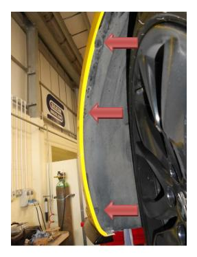
5. Moving to the underside of the vehicle. Undo the 5x T20 Torx screws.
