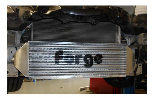
18. Using the 2x M6X16 Allen bolts and M6 penny washer supplied secure both ends of the intercooler to the original mounts.
