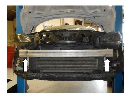
14. Using a Flat blade screwdriver undo the plastic screw on both ends of the air guides.
