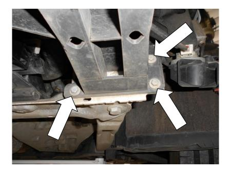
12. Unclip the connector from the centre of the crash bar, using a Flat blade screwdriver or similar tool remove the cable clips.
