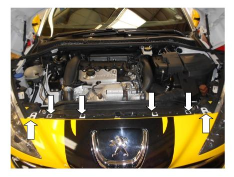
2. Using a flat blade screwdriver remove the 4x clips and undo the 2x T20 Torxs screws.
