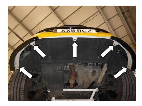
6. Using a Flat blade screwdriver remove the 2x clips on both sides.
