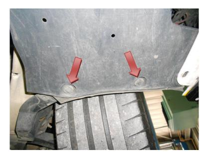
7. Using 10mm socket undo 3x bolts and undo the 2x plastic clips. Slide the under tray backwards and remove it from the vehicle. Store in a safe place away from the vehicle.
