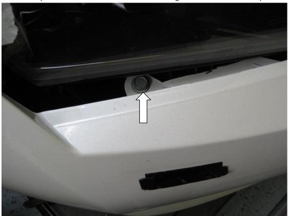
Push the sprung edge of the washer over to release it from the front face of the bumper, then push the washer through the hole.
