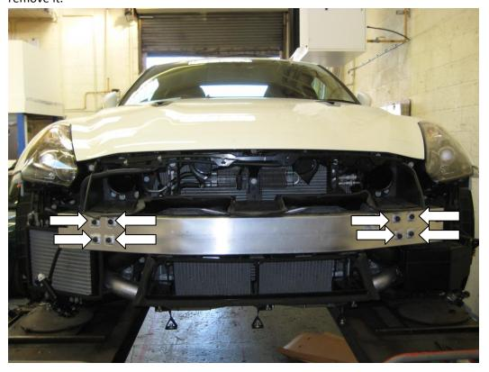
15. Remove the three supports that pass through the intercooler ducting noting their orientation on the brackets.
