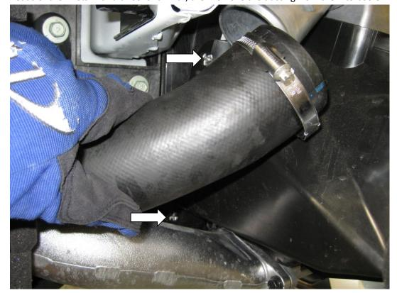
17. Remove the two bolts holding the intercooler inlet pipes to the chassis, the two bolts on the edges of the intercoolers (in the middle of the car) and one of the two top bolts of each intercooler (use a ratchet spanner), leaving one upper bolt to hold the intercoolers in.
