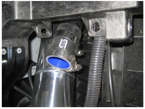
30. Fit the washer bottle pushing the filler neck on the tank into the silicon fitted in the last step. Fit using the three mounting brackets and bolts removed in step 15. Tighten the jubilee clip on the filler, reconnect the windscreen washer tube, and reconnect all of the wiring. Unfortunately the Forge washer bottle does not have provision for the level sensor which must be left disconnected – this won't bring on any warning lights.
