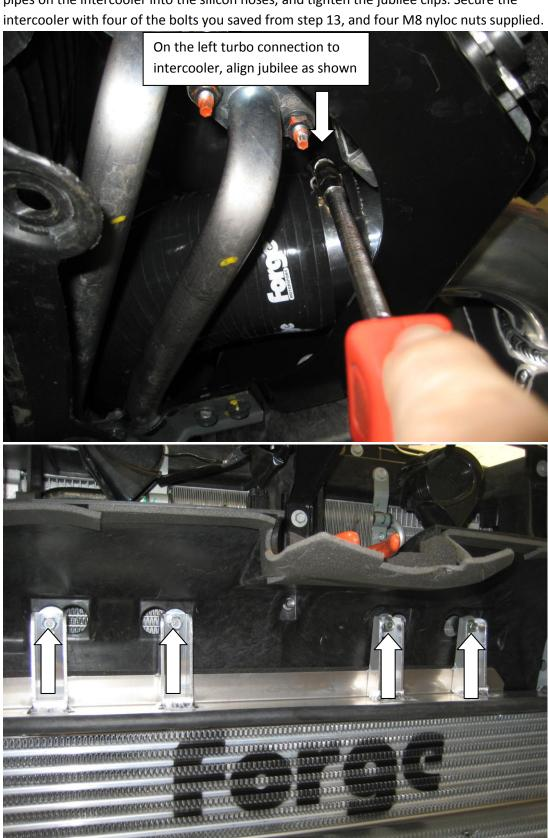
With the help of an assistant, push the bottom of the intercooler into the car to crush the rubber seal, and keeping the pressure on tighten with the last two bolts and M8 nyloc nuts.
