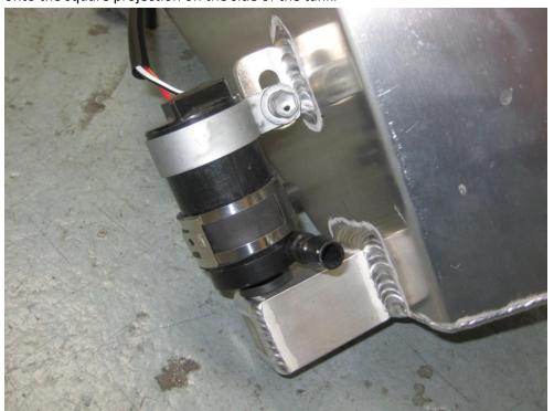
The washer pump is secured with the supplied cable tie.
