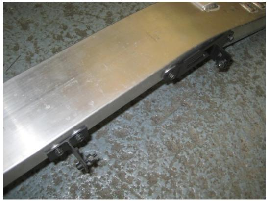
33. Refit the crash bar to the car, making sure the support brackets clear the edges of the cowl on the intercooler, and that the bolt heads on the brackets sink in to the rubber edging on the intercooler – this does also make the crash bar harder to refit however.
