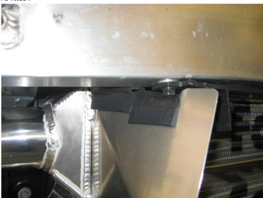
25. Lubricate the silicon hoses with silicon spray (dashboard cleaner works well) With the help of an assistant, offer up the intercooler to the car, sliding the lower left and upper right hard pipes on the intercooler into the silicon hoses, and tighten the jubilee clips. Secure the intercooler with four of the bolts you saved from step 13, and four M8 nyloc nuts supplied.
