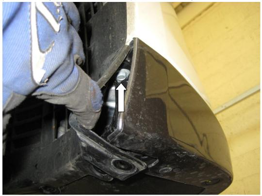
5. With the arch liner pulled out of the way, you will be able to easier access the other bolts holding the bumper to the wing. We found it easiest to use a long extension on a 3/8" drive to get onto the bolt.
