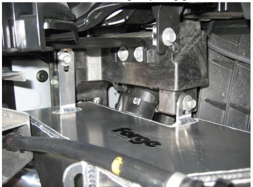
31. If you have headlight washers fitted, release the clip under the tee piece as shown below and cut approx 25mm of length from the hose but ideally measure on the car, then reconnect to the tee piece using the supplied 12mm jubilee clip (shown below with the pump missing).
