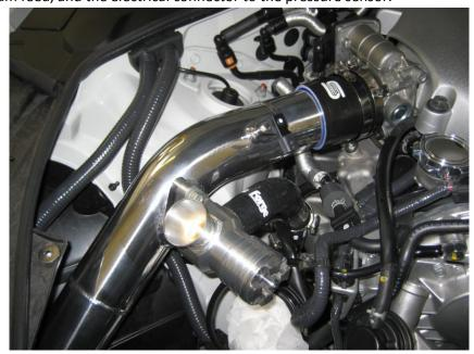
28. Take the remaining long hardpipe, and thread it up into the engine bay from the gap next to the intercooler. Add a straight coupler and two jubilee clips to each end of the pipe, then connect to the intercooler first. Ensure at least 25mm of hardpipe is left in each silicon joiner before tightening the clips. Refit the pressure sender and dump valve (again you may need to wait until you have refitted the airfilter).
