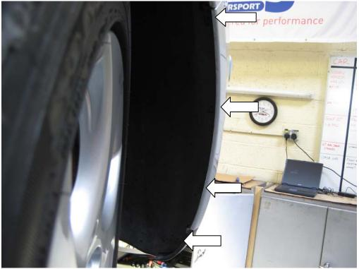
Now remove the single T25 screw that holds the edge of the bumper to the edge of the wing. This is very awkward to get at, though we had success with a  $\frac{1}{4}$ " drive T25 socket on a long  $\frac{1}{4}$ " extension.
