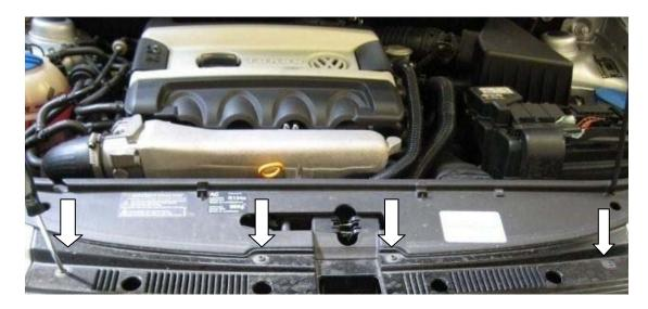
10. Back on the front of the bumper, behind where the foglight grills were, on the passenger side remove the external temperature sensor from the bumper by pushing the three clips in and pushing it back through the metal ring its housed in (see pic over page)
