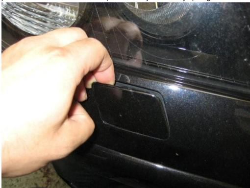
Once pulled out, simply pull the cover off by pulling it off the mounting lugs, one on each side – this is easy as the plastic is very flexible.
