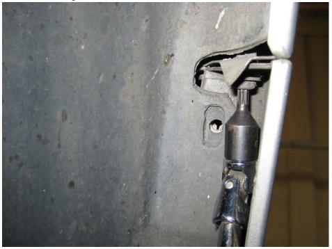
6. Working under the front of the car, remove the three T25 pan head screws on each side (shown in white below) that hold the undertray in place, and pull the undertray clear by pulling it towards the rear of the car.
