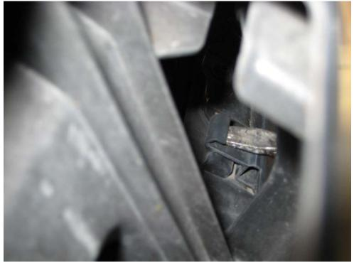
3. Remove both fog light covers at the bottom of the bumper, but note the drivers side one is retained by one phillips head screw (the passenger side has no screws). They can be removed by simply grasping the cover through the slats and pulling.
