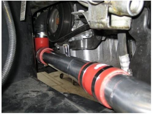
27. When you're happy with the location of the lower pipe, secure the bracket to the cotton reel using the supplied M6 nyloc nut and M6 small washer.
