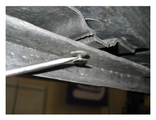
9. Back under the bonnet, remove the four T30 screws holding the top of the bumper to the slam panel. At this point the bumper can be quite loose, so be careful.
