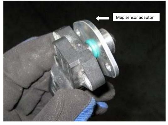
NOTE - the orientation of the MAP sensor when fitted in the pipework
