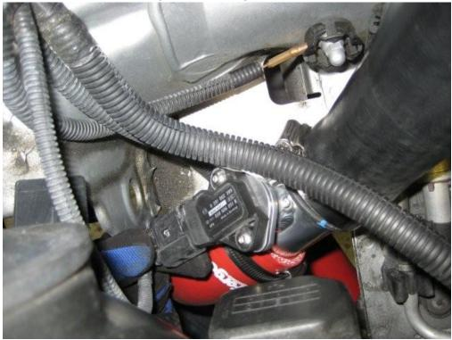
33. The intercooler should now be installed on the car, secured to the bumper and fully piped in with all hoses secure and all clips done up tight. Before continuing, you can test fire the engine to ensure it runs with no errors (you may get a warning light on the dash about the front foglights being disconnected however).
