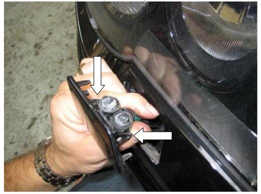
Now let the mechanism slide back into the bumper, and remove the T25 screw holding the mechanism to the back of the bumper.
