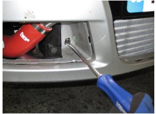
We found the easiest way to clip this back in was to use a large flat bladed screwdriver under the tab, push really hard on the end of the screwdriver to push the bumper back, then twist the head of the driver as the tab passes into the radiator surround. The tab should spring up and secure the bumper with a 'click'.
