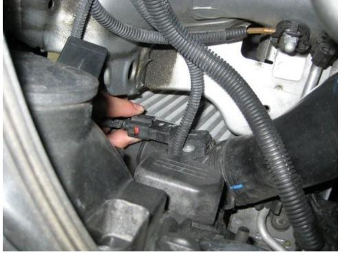
14. Move the hose clip from the lower intercooler hose, and remove the hose from the intercooler. Also remove the 10mm bolt holding the intercooler bracket to the chassis just above the lower pipe.
