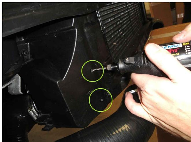
With the mounting holes drilled, position the Forge intercooler core in place and secure it using the supplied self-tapping screws and washers. If you encounter any resistance tightening the screws, please check the available depth of the hole to ensure that you are not touching the A/C condenser end tanks with the screws. Add washers as necessary if there is any conflict behind the holes.
