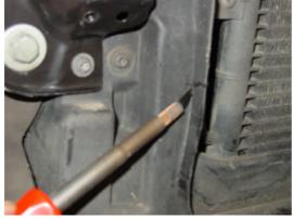
A small section of the front panel plastic edge will require trimming as per the picture, this is to allow the intercooler tube and pipe clearance. A craft knife or a strong sharp blade will be enough to cut through the plastic.
