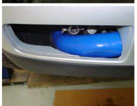
Before the front panel is refitted the lower grill aperture on the left hand side needs trimming to allow clearance for the lower intercooler hose as shown. This can be done with a craft knife or saw or hobby grinder. It is useful to use the replacement grill cover (supplied) as a template.
