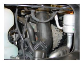
Completely remove the top hose from the intake manifold.
