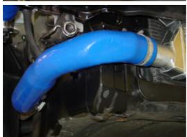
The lower silicone intercooler hose is now installed as shown, keeping the hose as close to the coolant radiator panel as possible, leaving a 2mm clearance. Ensure the hose clamps at both ends are secured.
