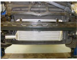
The bumper and intercooler assembly is now fitted to the vehicle using the 13mm bolts and T30 torx bolts that were removed from the original bumper.
