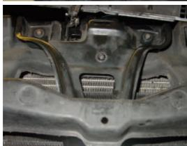
The bonnet (hood) locking panel brace needs removing (3 x T25 bolts) the lower portion of the bracket is cut
