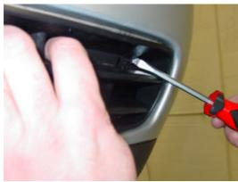
Remove the two lower air intake covers using a bladed screwdriver to pull down the upper locking tabs
