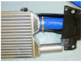
Next, assemble the new intercooler into the new crash bumper, as shown, securing the intercooler with the two 10mm bolts provided.
