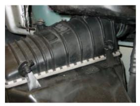
The front air guide can now be removed from the side mounted intercooler by gently prising the top clips free of the lugs and lowering off the lower securing bar. (Beware these clips are brittle)
