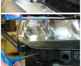
Remove the five T30 torx head bolts behind the grill panel that secure the front panel.
