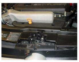
The front radiator grill can now be removed by pulling the top forward then lifting the grill upwards. There is no need to remove this completely as it is attached to the bonnet (hood) locking mechanism. Tilt upwards in order to gain access to the front panel securing bolts.
