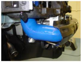
The silicone hose is now connected to the intake manifold and the clamps on both ends tightened.
