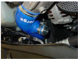
Insert the 25mm blanking plug into the top of the intake manifold hose and secure with the clamp provided. (This 25mm hose connection allows the relocation of the diverter valve with the optional "cold side relocation kit" if required.)
