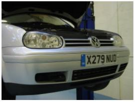
After ensuring that the vehicle is secured in a stationary position the front of the vehicle should be elevated so that both front wheels are off the ground using suitable lifting equipment (see manufacturers handbook for lifting points). Once elevated the vehicle should be "made safe" with secondary supports (axle stands) if necessary. The bonnet (hood) should be opened.
