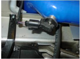
The MAP sensor (if fitted) from the original intercooler is removed and relocated into the silicone hose the screws provided. The sensor electrical connector is now refitted.
