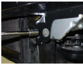
The front crash bumper is now removed by firstly removing the 13mm bolts and the T30 torx head bolts
