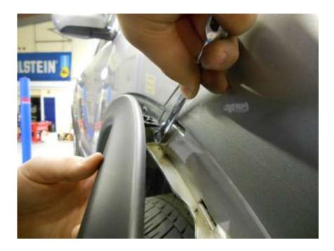
8. Carefully pull the bumper away from the clips that run up the bodywork and under the headlight. These are the last fixings holding the bumper to the vehicle.
