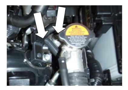
31. Fit the silicone S-bend to the outlet of the intercooler and secure with a suitable clip.
