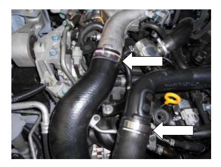
15. Undo the jubilee clip on the intercooler inlet and remove the standard hose.
