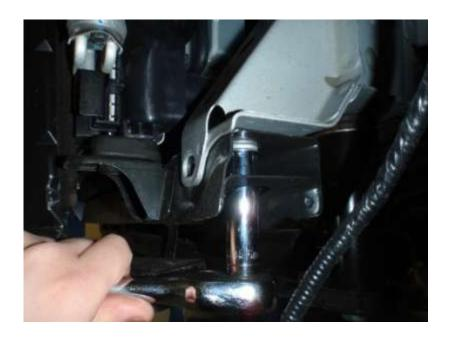
19. Carefully undo the vertical bolt in the lower beam at the intercooler end and the beam will drop away and the intercooler can be slid out of position.
