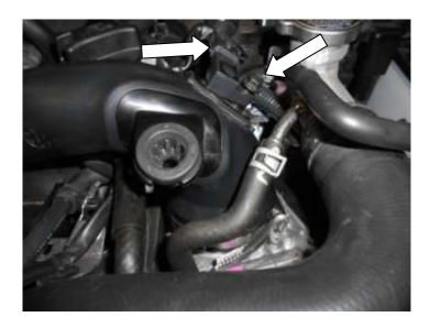
24. Using large pliers or a similar tool disconnect the pipes running to the dump valve.
