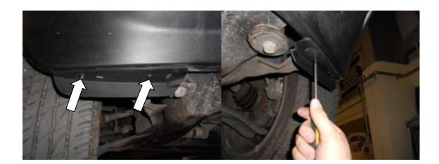
5. Using a flat blade screwdriver remove the plastic clip located at the front in both wheel arches.
