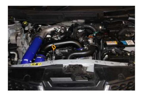
35. Check all hose clamps and fixings before refitting the bumper. Follow steps 9 to 2 in reverse to reassemble your vehicle. \*\* Please Note: Three different types of plastic clips are used to retain the bodywork on the Juke. They are of different length and reassembly will be difficult if put in the wrong locations.
