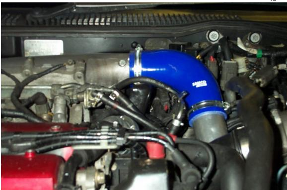
To the end of the metal pipe, attach a 45 degree bend. This will bring the end of the 45 degree bend nearly horizontal again. It should now be in a position between the inlet pipe (airbox to turbo) and the side of the inner wing. Attach the next longest metal pipe left, leave about 25mm of pipe showing, then attach the next 45 degree bend.
