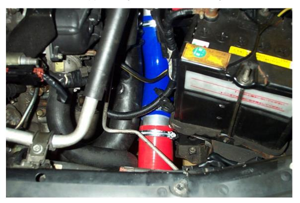
This bend needs to be placed under the small pipes for the air conditioner dual pressure switch (looks round from above, with a viewing glass on the top), and to the right of the radiator bottom pipe. This may be clearer:
