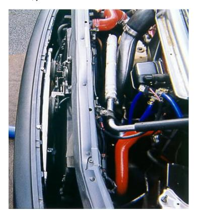
The two bolts for the top of the intercooler should fall in the area that is lipped on the top of the bumper bar, as seen in the picture above. Tighten (dont overtighten) for a secure fit.
