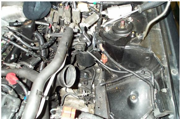
You may need to remove your dump valve (depending on type). Obviously we cannot cover the removal of every type of dump valve, as there are so many on the market. Suffice to say they are all easy to remove temporarily, to help fitting of the intercooler pipes. Remove all pipes from the dump valve and block them off temporarily. Shown below is removal of the Forge Motorsport dump valve
