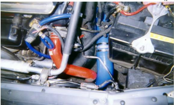
You should see a gap between the front of the chassis and the stabiliser bar (looks like a scaffold pole) to the right of the radiator bottom hose - this is the gap we are aiming for (it is JUST the right size). Attach the last longest metal pipe into the bottom of the 45 (leaving two very short metal pipes).
