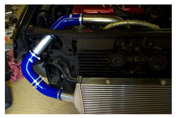
Check that the headlight remounts in its orifice. The sidelight connector will be very close to the metal pipe - this is nothing to worry about.
