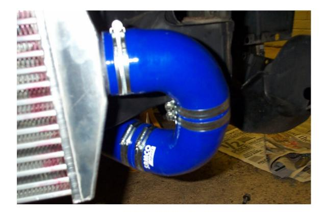
Put the next 90 on the outlet of the intercooler, angled down and slightly back. Connect the third 90 to the pipe from the engine bay using one of the metal connectors and trim if necessary. Use the last metal connector to join this 90 to the 90 from the intercooler. Tighten all jubilee clips.
