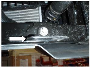
14. The brackets that were taken off with the metal pipe in steps 10 + 11 need to be replaced with the original bolts.
