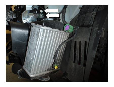
16. Undo the 10mm bolt and the 10mm nut holding the horn and intercooler on the passenger side, you will now be able to remove the complete intercooler unit by pulling upwards, with an even force to release the bottom pegs from the rubber grommets.
