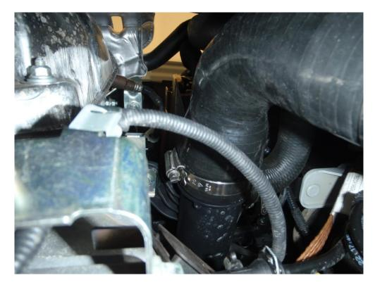
22. On the remaining silicon hose, loosely fit the 70 and 55mm jubilee clips. Push the large end of the hose onto the existing plastic pipe in the engine bay, and connect the other end to the joiner fitted in the last step. Tighten the jubilee clips. Now follow points 1-7 in reverse order and the installation is complete.
