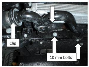
8. Now the bumper is off you will see a large black pipe which is connected to a rubber hose from the turbo, it has a 'use once' only clip this must be broken to remove. Undo the two 10mm bolts holding the pipe to the chassis and pull the clip out which is holding the hose to the pipe.
