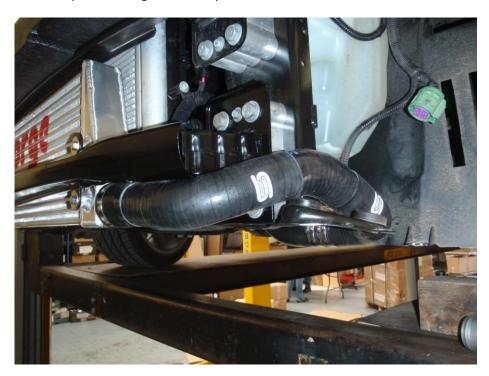
21. Push the long silicon hose onto the intercooler with a 55mm jubilee clip and do up in such a way that the bulky part of the clip is not on the bottom of the pipe becuase the intercooler sits slightly lower than stock. The silicon should be tight against the crash bar, going up and over the bracket of the old intercooler. Place the 45mm hose joiner supplied in the open end of the hose and secure with a jubilee clip.
