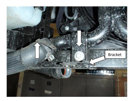
10.Looking at the back of the radiator you will see a large black pipe which is connected to a rubber hose from the passenger side intercooler, it has a 'use once' only clip this must be broken to remove. Undo the 10mm bolt shown, to remove the bracket keep to one side as this will need to be replaced once the pipe is removed.
