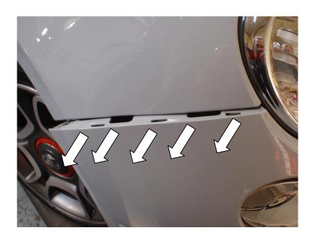
6. Pull the bumper away from the wing in the direction of the arrows with a firm but even pressure, taking care not to bend the bumper too much as this may crack the top edge.
