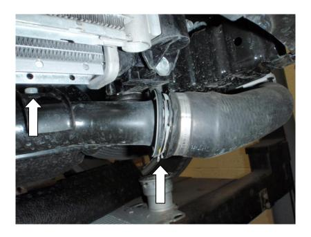
9. At the other end of the pipe, undo the last 10mm bolt, which secures the pipe to the chassis, using the 10mm ratchet spanner, and pull the clip out which is holding the hose to the pipe. This pipe is now free and can be taken off the car.
