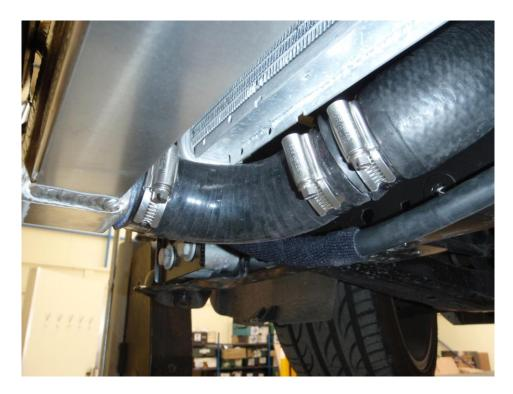
20. Push the coupler in to the stock rubber hose and tighten with a 50mm jubilee clip around the rubber hose. Put the two remaining 50mm jubilee clips loosely on the 90 degree silicon hose before installing, and then push the short leg of the 90 degree silicon coupler onto the intercooler and the long leg onto the coupler. Now tighten the clips on the silicon hose.
