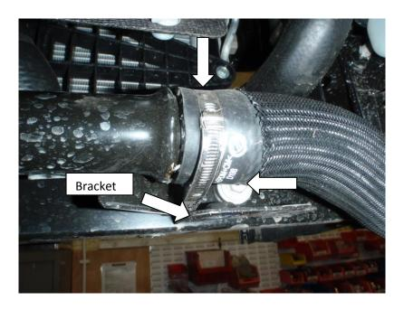
11.Looking at the driver's side of the pipe again the use 'once only' clip must be broken, remove the 10mm bolt and keep bracket to one side to be replaced after pipe is removed
