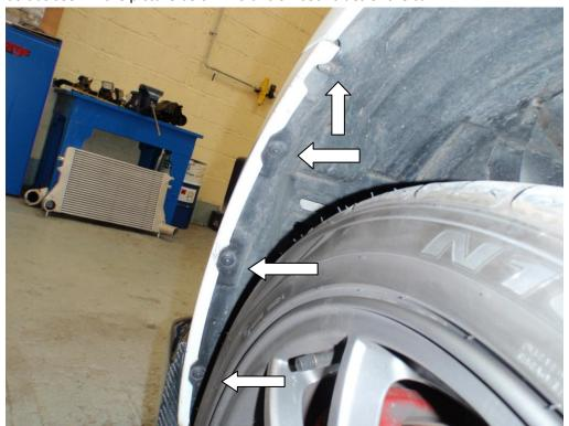
6. Remove 28 panel clips using a trim button removal tool, and the six 10mm bolts holding the undertray on, then remove.
