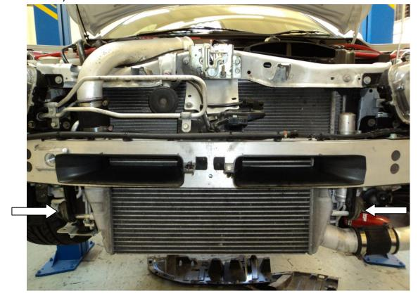
14. Once the intercooler is removed you will need to take out the metal insert and the rubber insert in the original intercooler and fit them into the new intercooler brackets provided.
