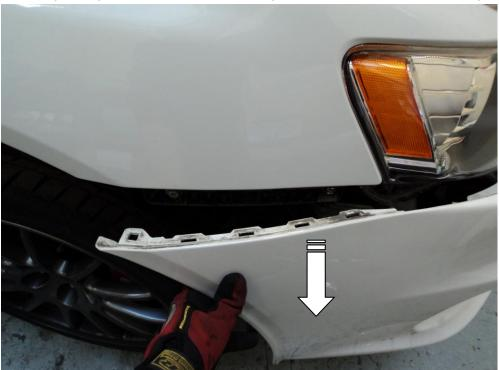
9. On the passenger side of the car using a trim button removal tool, remove the 3 panel pins holding the plastic shroud in place.
