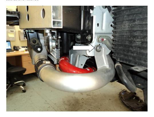
If you have the FQ360 model you will have to undo another two 12mm bolts as there are another 2 brackets holding the intercooler pipe in place as seen below.
