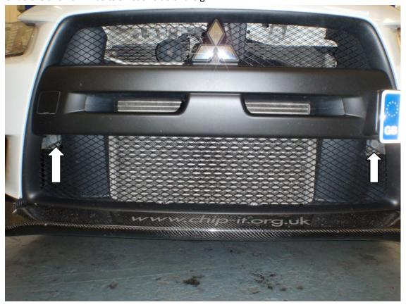
5. In the wheels arch, using a philips screwdriver undo the three plastic clips by unscrewing them 3/4 of the way out then removing the enitre clip. Now undo and remove the 10mm bolt as seen in the picture below. Do this on both sides of the car.
