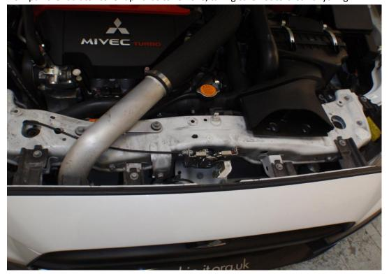
3. Remove the five 10mm bolts using a 10mm socket.
