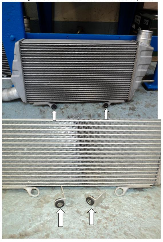
15. Fit the brackets in the same holes from where you removed the intercooler bolts from, using the two m8x15 bolts provided making sure to keep the brackets square when tightening with a 13mm socket and ratchet.
