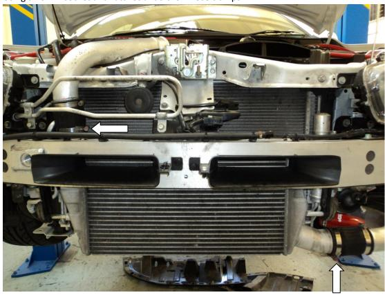
12. Undo the two 12mm bolts at the bottom of the intercooler using a 12mm socket and ratchet.
