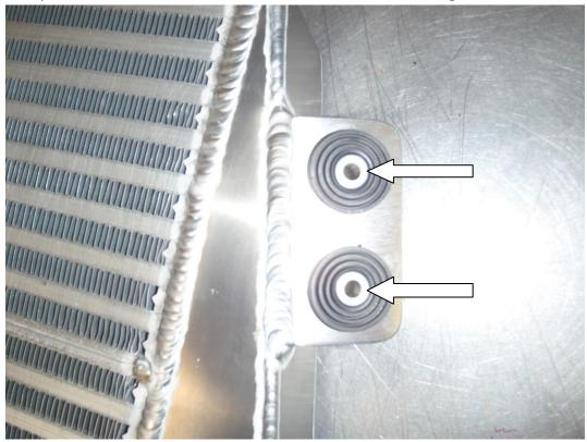
8. Place the crash bar over the intercooler and align the holes you have just drilled. Using the four M6x50 A/cap bolts along with the M6 washers, place them through the front of the crash bar and grommets on the intercooler.
