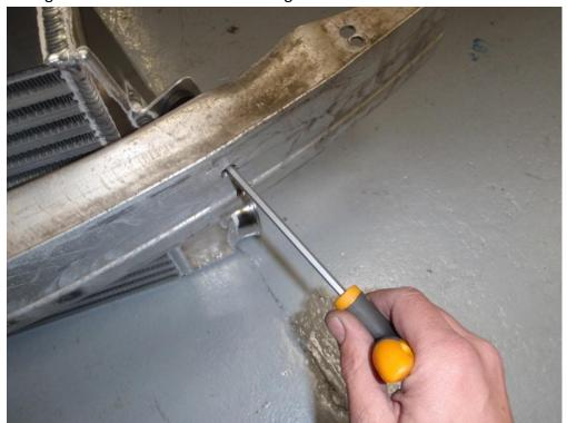
9. Once you have the bolts through, you will need to place the M6 penny washers and M6 nyloc nuts onto the end of the bolts and tighten.
