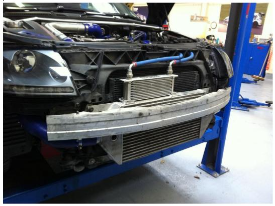
2. Using a 13mm spanner, undo the nut and bolt on each side of the crash bar.
