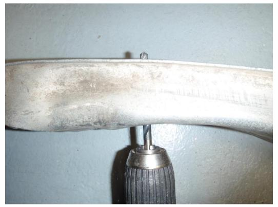
Turn the crash bar over and open out the holes on the front of the crash bar using a 13mm drill bit.
