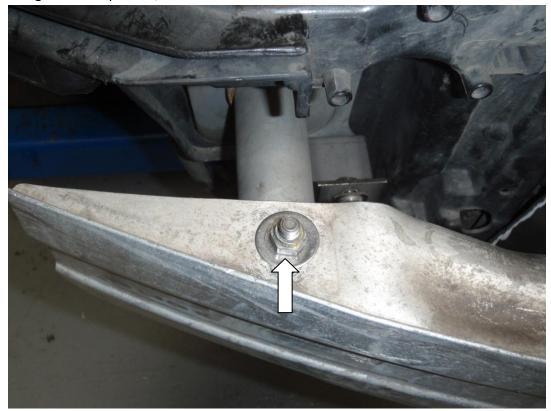
3. Mark back 6mm from the existing wholes on both top and bottom of the crash bar as seen below and drill using a 9mm drill bit.
