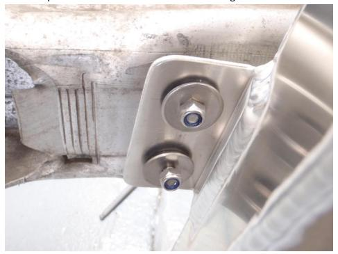
10. Now refit the crash bar using the new holes drilled in step 3 using the existing bolts and M8 penny washers supplied.
