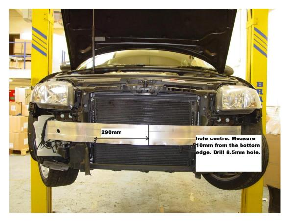
Fit the supplied brackets to the crash bar with the nuts & bolts supplied. Fit the intercooler to these brackets as shown. Tighten all the brackets and intercooler fixings once the intercooler is positioned centrally.
