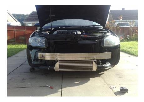
Depending on the original location of the ambient temperature sensor, it may require relocating to allow the intercooler to be installed. The sensor is removed from its existing bracket and refitted into the 13mm hole located on the side of the alloy intercooler bracket.
