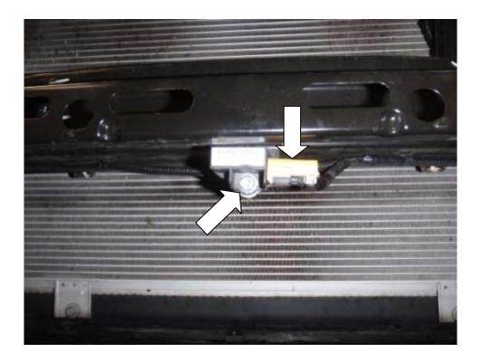
**13.** Starting on the inlet side of the OEM intercooler remove the sealing O-ring and install it on the corresponding side of the Forge intercooler. Repeat the process on the outlet side. **Failure to carry out this step will cause boost leaks within the intercooler system and loss of power.**
