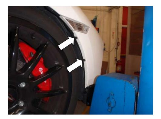
6. Carefully using a small flatblade screwdriver unclip the edges of the front bumper that extend above the front headlights. The retaining clips are accessible through the square holes in the top surface of the bumper; push the ends of the clips downwards to release them.
