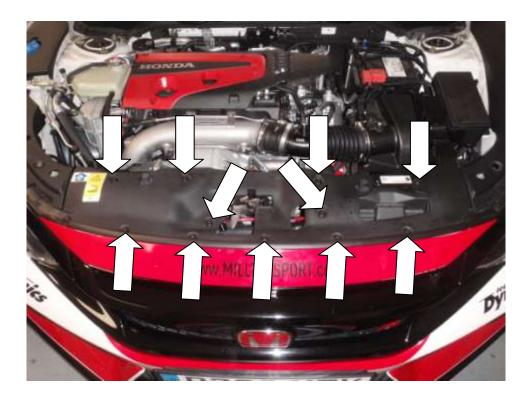
4. Remove the 5x plastic clips above each headlight. Take note of their type and position this will help with re-assembly. Carefully remove the rubber-edging strip.
