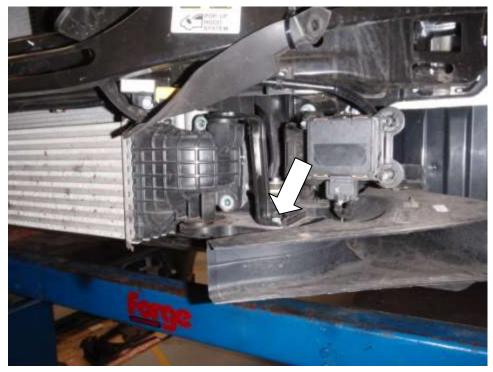
11. Carefully lift the intercooler off its lower mount to remove it from the vehicle.
