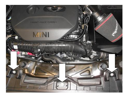
9. Unclip the sensors at each end of the crash bar and remove the foam crash bar cover. Note: <u>DO NOT SWITCH ON</u> THE IGNITION WITH THIS DISCONNECTED AS IT WILL CAUSE A WARNING LIGHT ON THE DASH WHICH CAN ONLY BE RESET AT A BMW DEALER.
