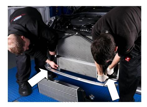
27. Pull the bottom of the intercooler forward and drop it down to release the radiator mounts.
