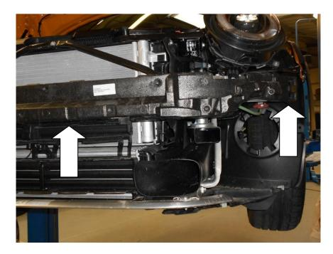
10. If fitted to your vehicle, unclip the wiring and using a T30 Torx driver undo the 2x bolts and remove the active air ducting.
