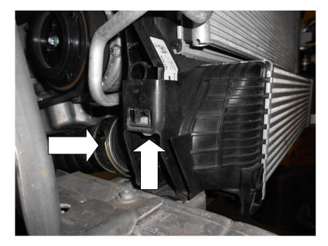
24. Moving to the underside of the vehicle using a flatblade screwdriver or similar tool remove the centre part of the intercooler clip.
