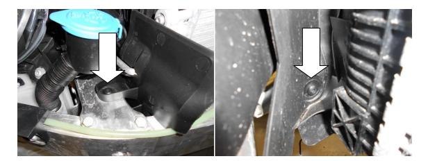
14. Using a 13mm socket and suitable ratchet undo 2x bolts on either side of the crash bar. Pull the crash bar forward and remove it from the vehicle.
