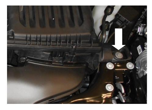
20. Using a 10mm socket and suitable ratchet remove 1x bolt.
