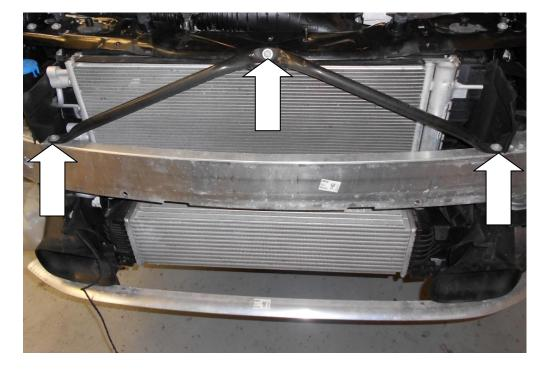
11. Undo 3x T30 Torx screws and remove the front brace.
