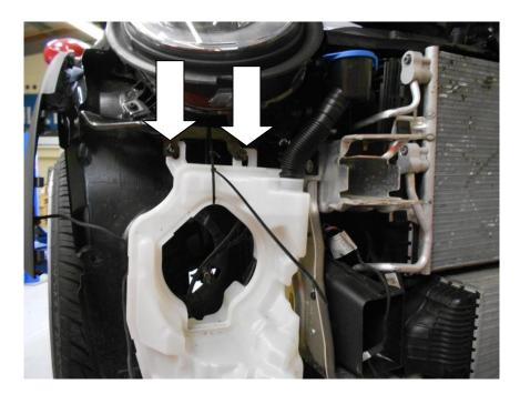
Using a flat blade screwdriver or similar remove the 2x clips inside the wheel arch. Using T27 Torx driver undo the 1x screws. Lift the duct upwards to release it and remove it from the vehicle.
