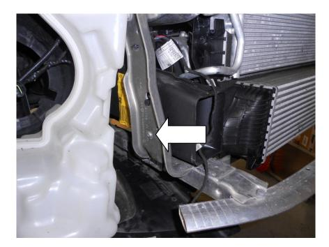
19. Undo the 5x T30 Torx bolts around each bonnet catch; do not fully remove the bolts.
