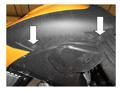
4. Using 8mm socket and suitable ratchet undo the 1 off screw inside each wheel arch. Rotate the access panel inside the wheel arch and unclip wiring to the back of the fog light on both sides.
