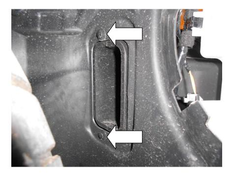
16. Using T27 Torx driver undo 1x screw and unplug the temperature sensor. Lift the duct upwards to release it and remove it from the vehicle.
