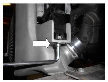
32. Re-connect both intercooler hoses. Ensure that the spring clips are fully released and have fully engaged in the recess in the CNC coupler. If these are not correctly installed they may come off during normal driving.
