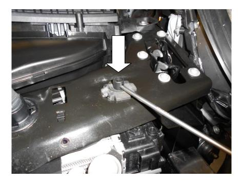
23. Undo the 2x T30 Torx screws on either side of the intercooler. Using a flat blade screwdriver or similar tool carefully release the spring-clips and disconnect the hose at each end of the intercooler.
