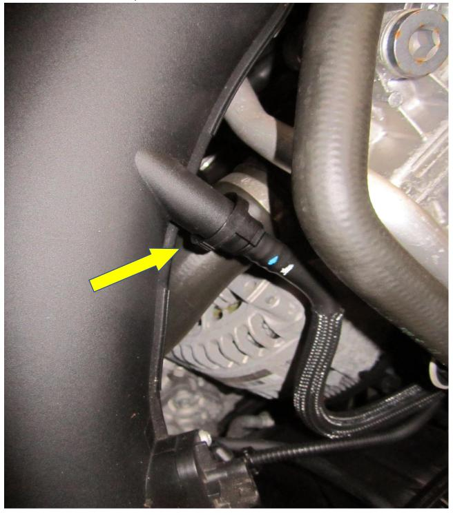
**11**. The longer inlet pipe can now be removed.
