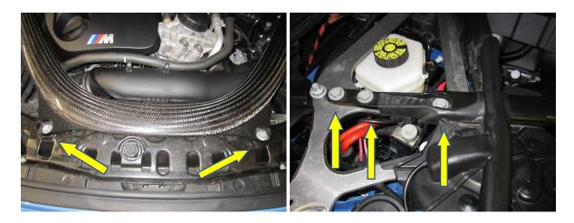
6. Undo the 10mm fastener that holds the charge cooler expansion tank to the strut brace.
