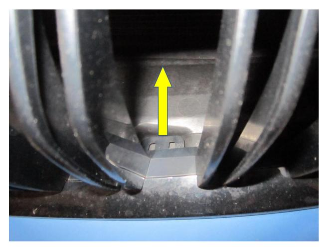
**13**. With the kidney grills removed, the front air scoops can be bolted into position by using a 13mm spanner and a 8mm Allen key.
