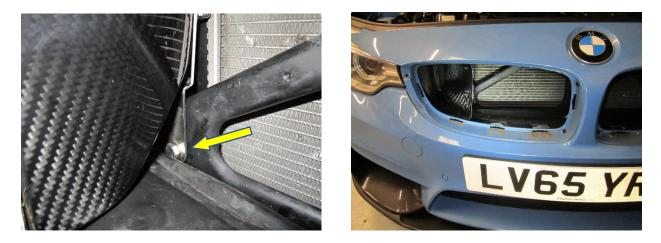
14. Remove the fastener arrowed below with an 8mm socket.
