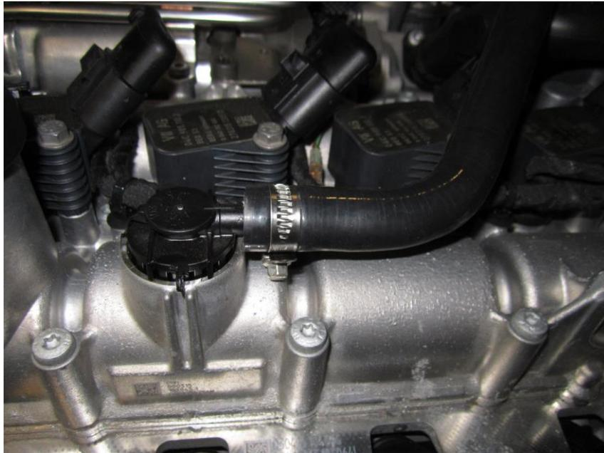
7. You can now tighten the final hose clamp that connects your silicon hose to the plastic turbo inlet hose. **AGAIN TAKE CARE TO NOT OVERTIGHTEN THE HOSE CLAMP AS YOU COULD CRACK THE PLASTIC.**
