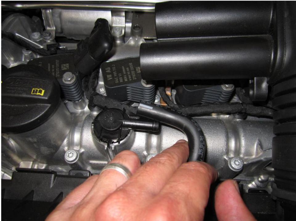
4. Now by pulling upwards in a sharp movement remove the airbox .
