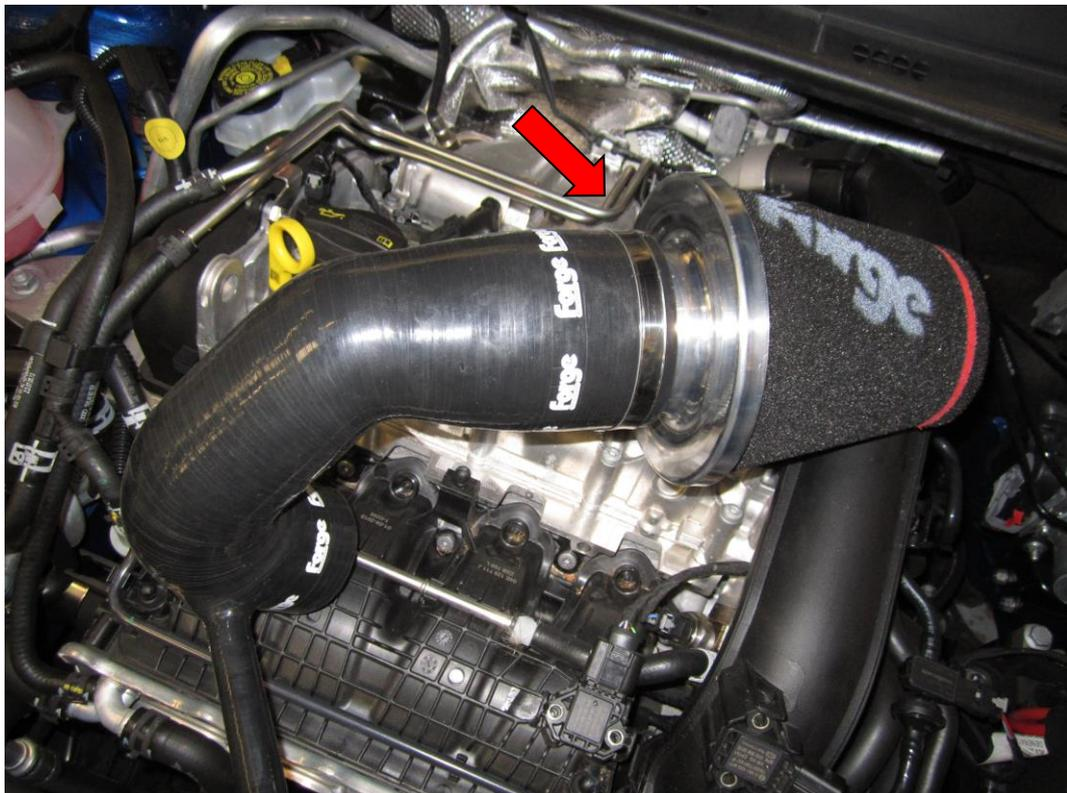
6. Fit the new silicon inlet hose into position and connect the breather pipe to the rocker cover, then tighten the hose clamp.
